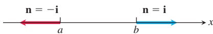
FIGURE 16.84 The outward unit normals at the boundary of [a, b] in one-dimensional space.
