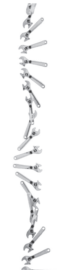
FIGURE 6.44 A wrench gliding on ice turning about its center of mass as the center glides in a vertical line. (Source: Berenice Abbott/ScienceSource)
