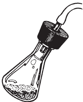
FIG. 9.6 Drying a solid by reduced air pressure.
