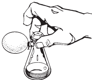
FIG. 25.8 Apparatus for macroscale Brown hydrogenation.
