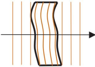
**Windows** are used in transmission, thin sections bend, and bending has a negligible effect on TWD, *especially* in thin sections. TWD is the preferred specification for windows unless the quality of a surface reflection is a functional requirement.
