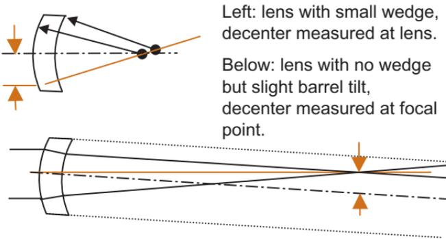
Wedge or **beam deviation** angle are preferable to centration tolerances in this type of optic. These parameters are more easily measured in the shop and more closely related to optical performance than centration is.
