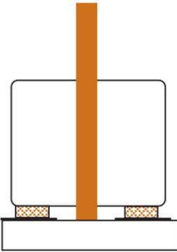
A Nd:YAG laser rod, for example, is set into a heated, waxed bore in the center of a steel block, one end of the rod protruding to contact a reference plate while the undoped outrigger feet stand on shim material.
