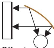
Off-axis parabolic null
