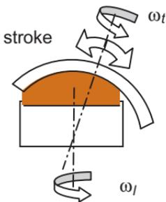
The rigid tool,  $\sim 2\times$  the diameter of the lens, is faced with a plastic pad. Using high pressures and rotation rates of  $\sim 1000$  RPM, polishing time from a high-quality modern generator is only a few minutes. The lens is supported in back by a pressurized bladder to minimize sagging, and force-fed slurry is refrigerated to minimize heat distortion. Although not optimal, with special tooling such machines can approach hemispherical curves.
