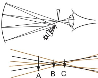
The **Foucault knife-edge test** is the classic **slope evaluation** method, in which the caustic is intercepted by a blade directly in front of the eye. It is surprisingly sensitive and requires no expensive gear. While only qualitative for high- and mid-spatial-frequency slopes, quantitative
