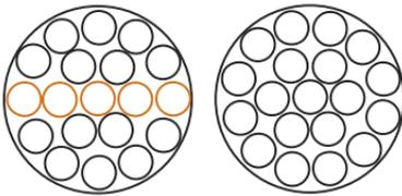
A quick method to determine flat block pattern is to lay out parts across a block diameter with  $\phi/10$  spacing between and count how many fit; then use the table below.
