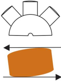
In general, thicker parts are easier to fabricate than thin parts. Exceptions include thick-edged strongly convex lenses (due to sparse **block** packing) and tall flat parts to be **double-lapped** (due to a tendency to rock between the laps).
