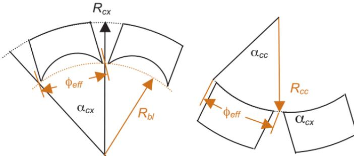
It should be clear from the above that thick lenses with steep convex radii can only be worked singly.
