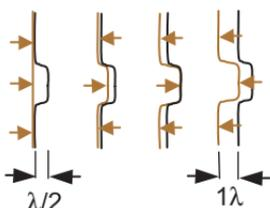
One fringe spacing *always* represents one wave of optical path difference (OPD) at the plane of interference.
