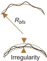
**Radius:** radius of the RMS best-fit sphere to a surface or wavefront.
