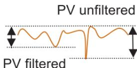
the greatest positive deviation and the greatest negative deviation from a desired function such as a best-fit sphere, or “flatness.” It is familiar and easy to evaluate, but can be highly influenced by small areas
