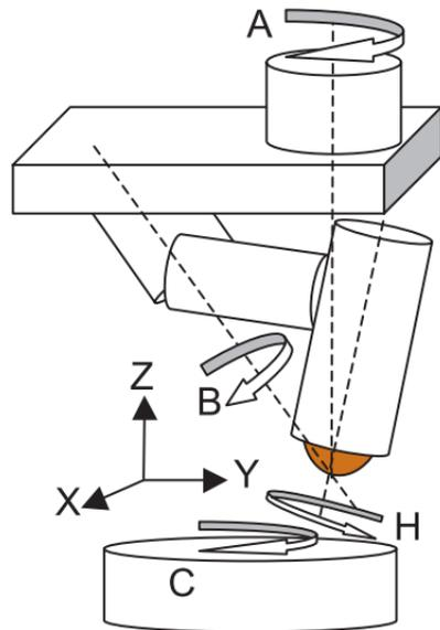
When the contact patch does not include the center of rotation of the tool, the removal function is nearly spherical. **Precession** about axis  $A$  eliminates directional lay.
