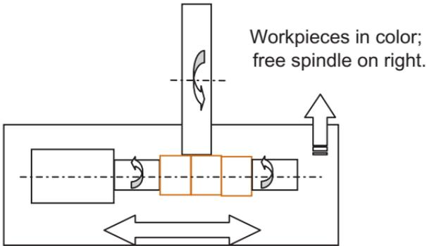
The reciprocating motion spans all workpieces and maintains the abrasive wheel as a true cylinder. Machine stops set the reciprocation stroke and finish diameter.
