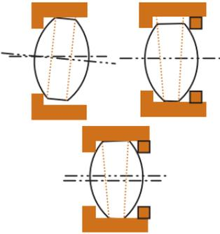
Multiple-lens systems are held to accurate alignment and spacing by mounting in cells and stacking in barrels. Centration is only achieved through consistency between element **datum** systems and cell datum systems.
