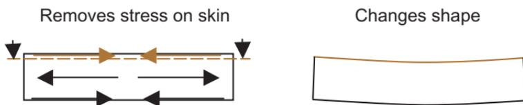
The Twyman effect: Grinding and lapping induce surface compressive stress, decreasing with abrasive size below 50  $\mu\text{m}$ , reducing gradually over time, and being relieved by etching or polishing.
