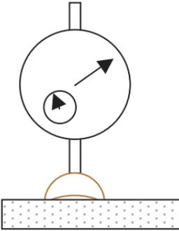
**Drop gauge**, as colloquially known, is a hard-mounted linear probe contact gauge used to measure small excursions of the gauge pin or to compare two arbitrary positions. With potential accuracy to  $0.5\ \mu\text{m}$ , this type of gauge is useful for measuring wedge, height, and center thickness.
