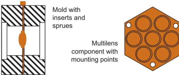
Plastics offer high impact resistance and low specific gravity ( $0.2\text{--}0.5\times$  other optical materials.) Due to plastics' high coefficients of expansion, shrinkage in the mold must be considered in the cavity design to minimize distortions. Due to high viscosity and chain molecules, **birefringence** is prominent. Careful material selection, cavity margin and sprue design, and process development help minimize these concerns.
