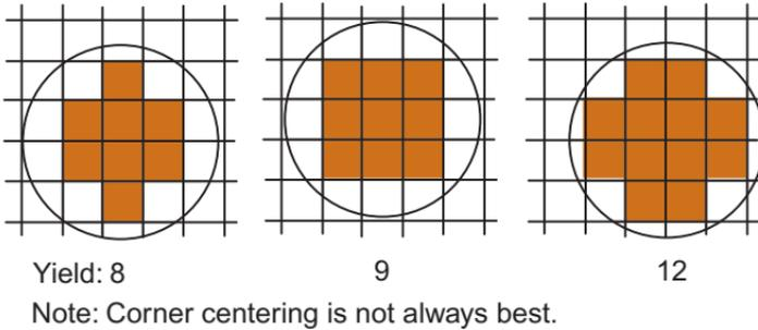
To minimize yield loss to kerf width on small parts, narrow blades are used. These are inherently more flexible and fragile. Proper blade alignment, support, balance, coolant flow, and feed rate are critical. A square cover piece helps guide off-center cuts.
