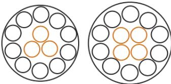
The best packing could have one, three, four, or even five parts in the inner zone. Subsequent zones should be spaced in circles.
