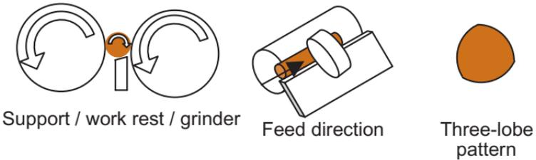
The rod is introduced to the machine at one end. The angle between the support wheel and grinding wheel causes the rod to “walk” down its length and exit on the opposite end.
