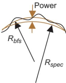
**Power:** difference between the *specified* sphere and the best-fit sphere. Cylindrical power is measured along its axis. Power should not be applied to aspheres. For non-circular areas, apertures must be carefully defined.
