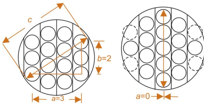
The tool, when loaded with workpieces, must balance on the areal center of the workpieces as well as on the spindle pin, which may need to be decentered.
