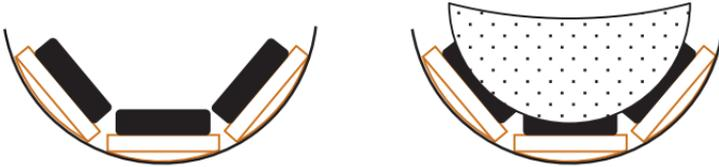
The pitch should be a few millimeters thick at its thinnest point and relatively equal in the inner and outer zones.
