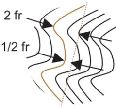
Fringe patterns for nonspherical surfaces change shape with tilt.
