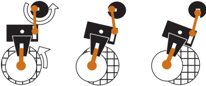
**Warning:** If the pin directly passes over the axle, all of the forces suddenly reverse, and the spindle jumps.
