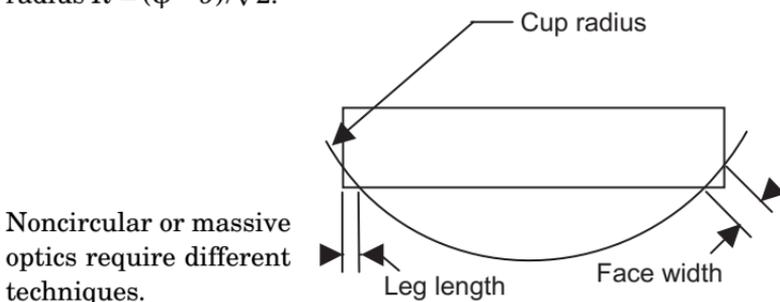
Rebeveling during fabrication is often preferable to making a larger bevel at the outset; producing a bevel by hand takes time proportional to its *volume*, not its width.
