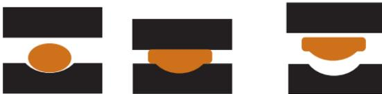
Glass manufacturers have created families of glass with low **transition temperatures ( $T_g$ )**, specifically designed for compression molding. Still, there is thermal contraction upon cooling below  $T_g$ , so the final result does not exactly match the mold. Precision molders model this in advance and adjust the mold surfaces to compensate. The optics are slowly **annealed** after molding.
