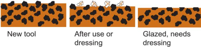
When machine loads increase or the lapping rate decreases, dress the tool briefly against a grinding stick to expose fresh abrasive.
