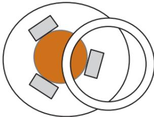
Left: Top view of the Blanchard mill with the workpiece in color.
