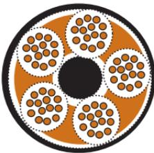
Top view: Lower lap in color, ring and sun gear in black, carriers in white. Upper lap (matching lower) is removed. Parts should be periodically flipped over and shuffled to maintain uniformity.
