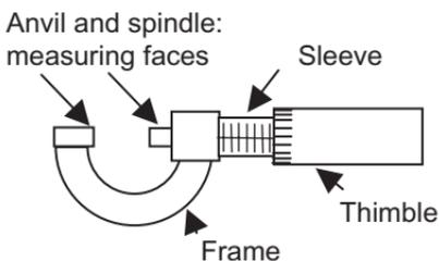
**Anvil micrometers** are the basic tool for linear measurement. Minimum calibration consists of checking the reported thickness of several different **gauge blocks** across the micrometer's full range of measurement,
