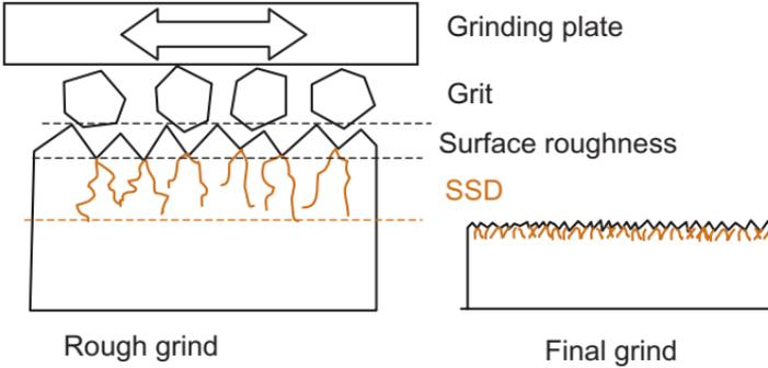
Remaining fractures are known as **subsurface damage (SSD)** and can safely be assumed to be less than  $1.4\times$  the grit size. It is good practice to remove  $2\times$  the previous grit size.
