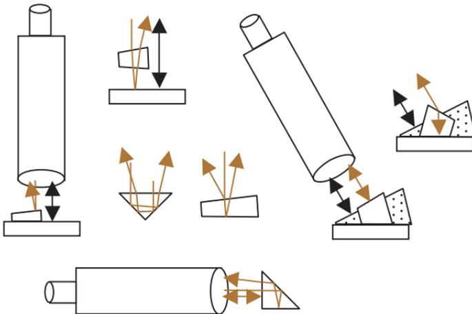
This figure displays a small fraction of the tests and configurations possible with a single autocollimator.
