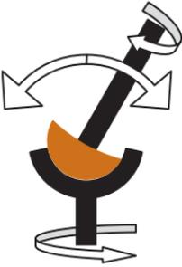
**Stick machines** generally have six or more rotating spindles and reciprocating arms ganged together in identical motion. The overarm motion is an arc concentric with the lap's center of curvature. The stick and lens may freely rotate or be driven counter to the lap.
