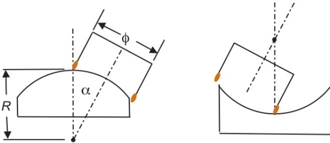
Convex (left) and concave (right) generating geometries.
