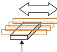
**Gang saws** come in two types: Parallel rotating wheels in a precision saw, or reciprocating parallel straight blades (like a hacksaw), for making multiple simultaneous cuts.
