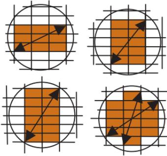
Compare the usable area of the parent to the pattern diagonals (counting the saw kerfs) for each of four pattern centers: corner, vertical face edge, horizontal face edge, and part center. The best arrangement is dimension dependent. The sketch here shows yields of 9, 10, 12, and 14, depending on the starting position.
