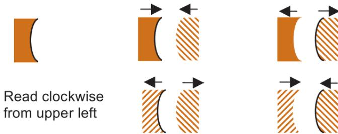
Alternatively, the submaster can be replaced with a directly produced negative master. This variant is particularly helpful where the finished part (and by extension its original master) is a convex asphere that would be difficult to test directly. Thin-film coatings can be applied to the submaster.
