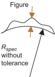
**Figure:** overall physical shape, as compared to specified geometric ideal. If no tolerance is given to the radius, then figure includes both power and irregularity. If the radius is separately toleranced, figure is equivalent to irregularity, but the best-fit sphere must also be within the radius tolerance.
