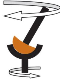
To maintain equal removal across entire surface at successive abrasive grains, the lap radius has to chase the shrinking lens.
