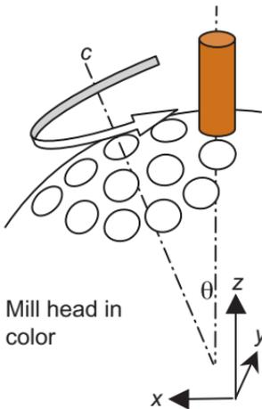
Monolithic spot tools are machined on a five-axis mill. Errors along the  $y$  axis cause uncorrectable wedge in all parts.  $x$ - or  $\theta$ -axis errors cause relative wedge in that row.  $Z$ -axis errors affect that part's thickness. Burrs on seats affect thickness and wedge. Fortunately, there are simple diagnostic tools using only ground glass coupons, dial gauge, and pencil.<sup>5</sup> Each tool has an ideal part thickness, and accepts but one diameter.
