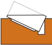
Because acute angles are fragile (and sharp!) it is a good plan to leave original faces from the **blanks** as bevels, when possible.
