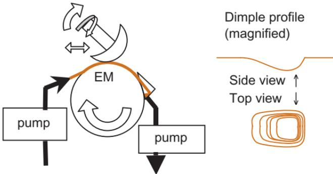
A notable feature of MRF<sup>®</sup> is that polishing is driven by shear forces—the pressure term of Preston’s equation in conventional polishing is of little consequence. When coupled with on-machine interferometry and CNC control, this feature enables rapid convergence on any desired figure or transmitted wavefront from any (prepolished) starting shape. Subsurface damage is essentially eliminated, resulting in a high laser damage threshold. Print through is minimized.
