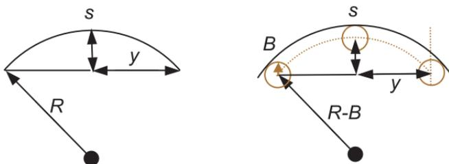
When using a **spherometer** with ball feet:
