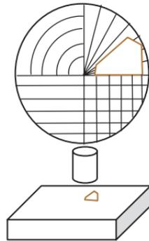
Vision systems apply automatic feature recognition. Edges, circle centers, diameters, etc. and their relationships are identified in accordance with geometric dimensioning and tolerancing (GD&T) rules.
