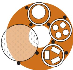
In this top view, the three annuli are work rings containing four small rounds, one large round, and three rectangles, respectively. The large circle on the left is the **conditioner plate**. The small black circles are fixed roller wheels that keep the conditioner and work rings from rotating with the lap.
