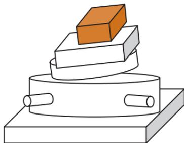
Nonlinear crystal oriented on goniometer atop backing glass, ready for wire sawing or surface grinding
