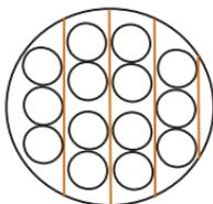
Once the slot layout is chosen, the optician may choose to space the parts within the slots to make a smoother outer perimeter.
