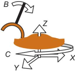
Common motions include  $X$ ,  $Y$ , and  $Z$  as with standard mills, plus  $C$  for workpiece rotation, and  $B$  for tool head tilt about  $Y$ .
