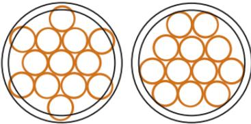
A similar approach works for coring from a circular parent with only two options: hexagonal with one part or three parts in the center.
