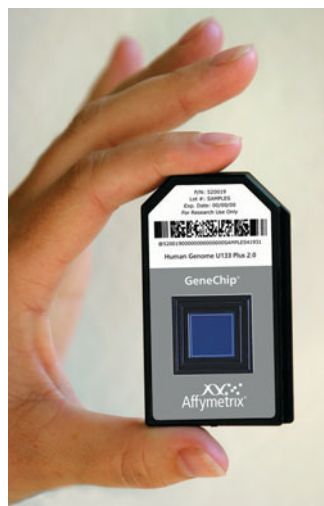
◀ Figure 18.4 A human gene microarray chip. Tiny spots of DNA arranged in a grid on this silicon wafer represent almost all of the genes in the human genome. Using this chip, researchers can analyze expression patterns for all these genes at the same time.
