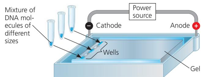
**(a)** Each sample, a mixture of DNA molecules, is placed in a separate well near one end of a thin slab of agarose gel. The gel is set into a small plastic support and immersed in an aqueous, buffered solution in a tray with electrodes at each end. The current is then turned on, causing the negatively charged DNA molecules to move toward the positive electrode.
