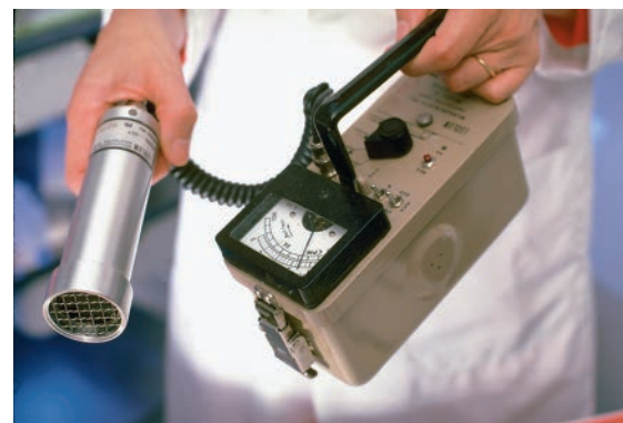
▲ FIGURE 20.8 Geiger-Müller Counter When ionizing radiation passes through the argon-filled chamber, it ionizes the argon atoms, giving rise to a brief, tiny pulse of electrical current that is transduced onto a meter or into an audible click.
