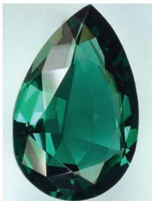
▲ Ruby and Emerald The \text{Cr}^{3+} ion is responsible for both the red color of ruby and the green color of emerald.
