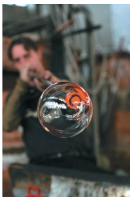
▲ Glassblowing involves blowing air into a hot piece of glass to form spherical shapes.
