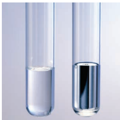
▲ FIGURE 11.19 Menisci of Water and Mercury The meniscus of water (on the left) is concave because water molecules are more strongly attracted to the glass wall than to one another. The meniscus of mercury is convex (on the right) because mercury atoms are more strongly attracted to one another than to the glass walls.
