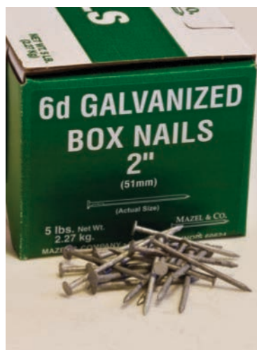
◀ In galvanized nails, a layer of zinc prevents the underlying iron from rusting. The zinc oxidizes in place of the iron, forming a protective layer of zinc oxide.
