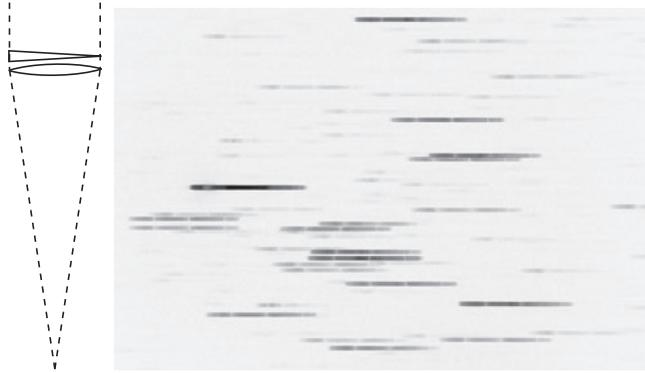
Figure 10.10 (Left) Schematic illustration of an objective prism. (Right) An objective prism image of the Hyades (courtesy of Dean Ketelsen). The Balmer absorption lines can be easily seen. This technique can also be used to find emission lines such as [O III] 495.9, 500.7 nm. For color version of figure, see plate section.
