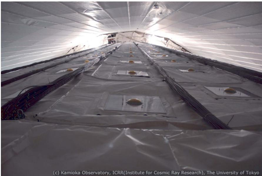
Plate 14.10 The outer portion of the Super-K detector with outward-looking PMTs.
