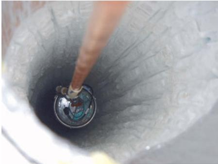
Plate 14.18 Photomultiplier being lowered down into a 2 km hole in the antarctic ice. Courtesy of IceCube/NSF.
