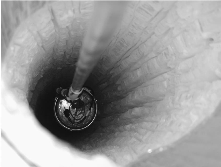
Figure 14.18 Photomultiplier being lowered down into a 2 km hole in the antarctic ice. Courtesy of IceCube/NSF. For color version of figure, see plate section.
