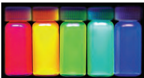
Figure 14.1-13 Photoluminescence from colloidal CdSe quantum dots (with oleylamine surface capping molecules) dispersed in n -hexane, in response to ultraviolet excitation at \lambda_o = 365 nm. Quantum-confinement effects allow the emission color to be tuned with quantum-dot size (courtesy Dong-Kyun Seo, Arizona State University).
