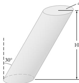
FIGURE 10 Cylinder inclined at an angle  $\theta = 30^\circ$ .
