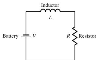
**FIGURE 1** Current flow approaches the level  $I_{\max} = V/R$ .
