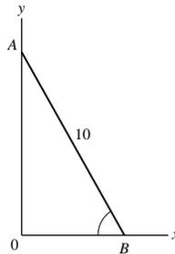
As the ladder slides down the wall, the  $x$ -coordinate of  $A$  is always zero and the  $y$ -coordinate is  $y = 10 \sin \theta$ . The parametric equations for the path followed by  $A$  are thus
