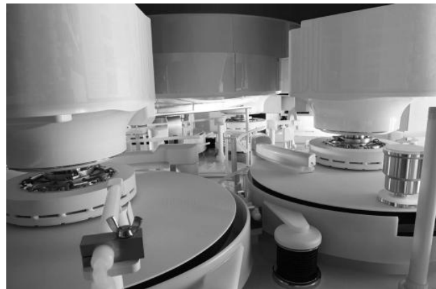
Figure 3.20 CMP process shown schematically on the left with an actual machine on the right, (the Applied Materials Reflexion CMP tool). Photo courtesy of Applied Materials, Inc.
