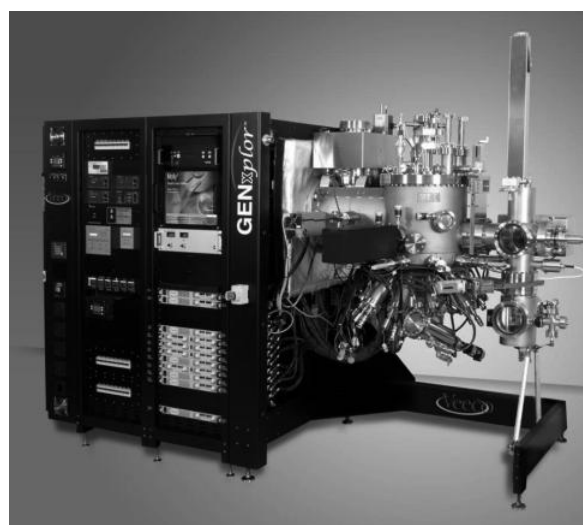
Figure 10.36 (Left) Schematic of an MBE chamber, showing the source effusion cells, RHEED analytical monitoring of layer thickness and other ports. (Right) A commercially available Veeco MBE system, showing various stainless steel ports and chambers. Photo courtesy Veeco Corp., used with permission.
