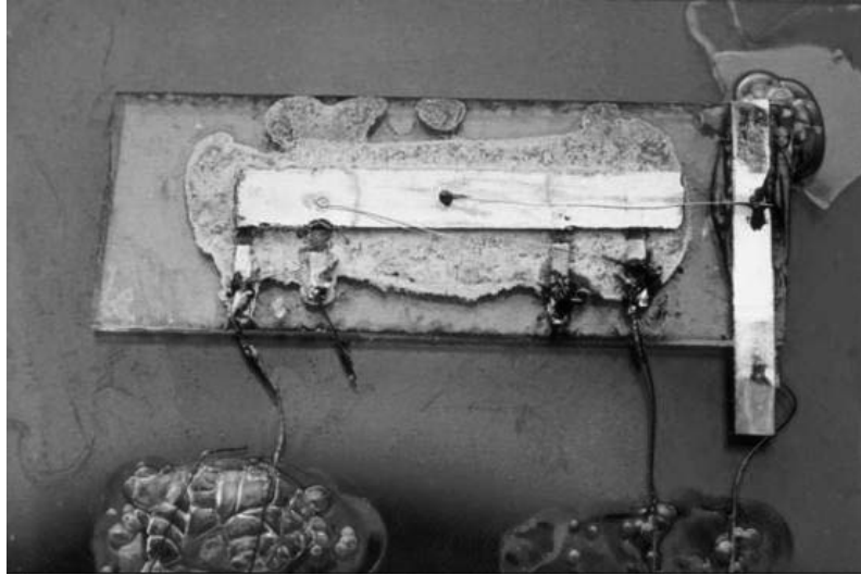
Figure 1.8 First integrated circuit constructed by Jack Kilby in 1958. Photo courtesy Texas Instruments.
