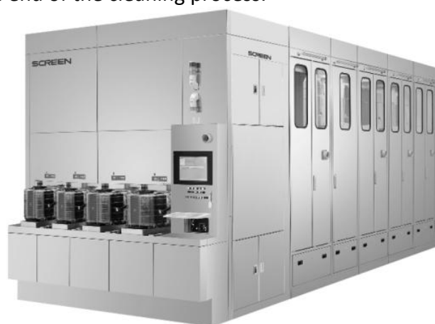
Figure 4.12 Left: A simple cleaning station. Wet chemical cleaning baths are in the sinks. The robot is loading a cassette of wafers into a spin dryer. Photo courtesy Ruth Carranza. Right: a modern fully enclosed automated system for RCA cleaning. Photo courtesy SCREEN Semiconductor Solutions, reprinted with permission https://www.screen.co.jp/spe/en .
