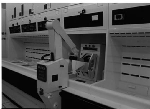
Figure 4.12 Left: A simple cleaning station. Wet chemical cleaning baths are in the sinks. The robot is loading a cassette of wafers into a spin dryer. Photo courtesy Ruth Carranza. Right: a modern fully enclosed automated system for RCA cleaning. Photo courtesy SCREEN Semiconductor Solutions, reprinted with permission https://www.screen.co.jp/spe/en .
