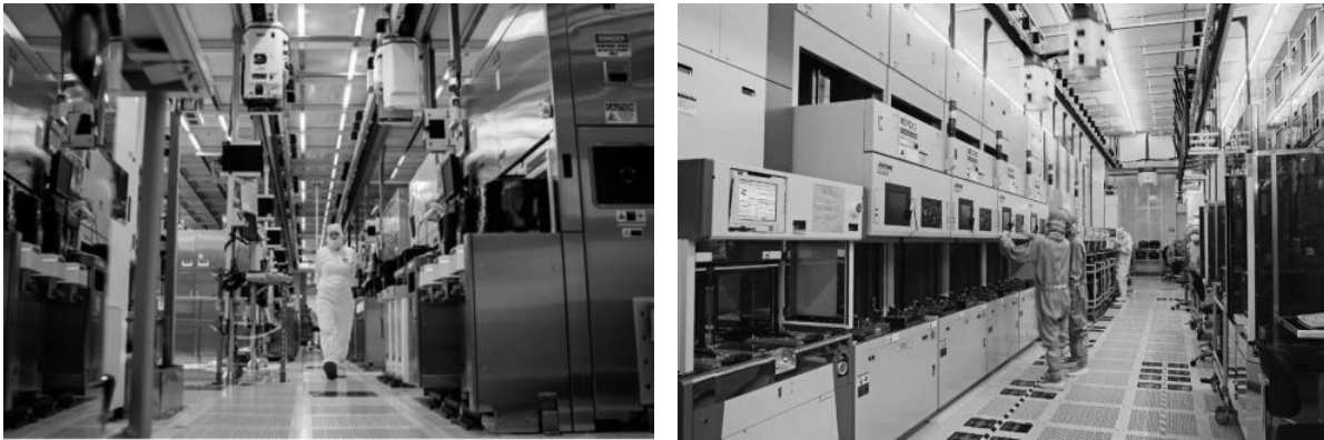
Figure 4.7 Modern silicon chip manufacturing facilities. The wafers are carried in sealed containers on the ceiling tracks from machine to machine. Left photo courtesy Intel, right photo courtesy Taiwan Semiconductor Manufacturing Co., Ltd. (TSMC).
