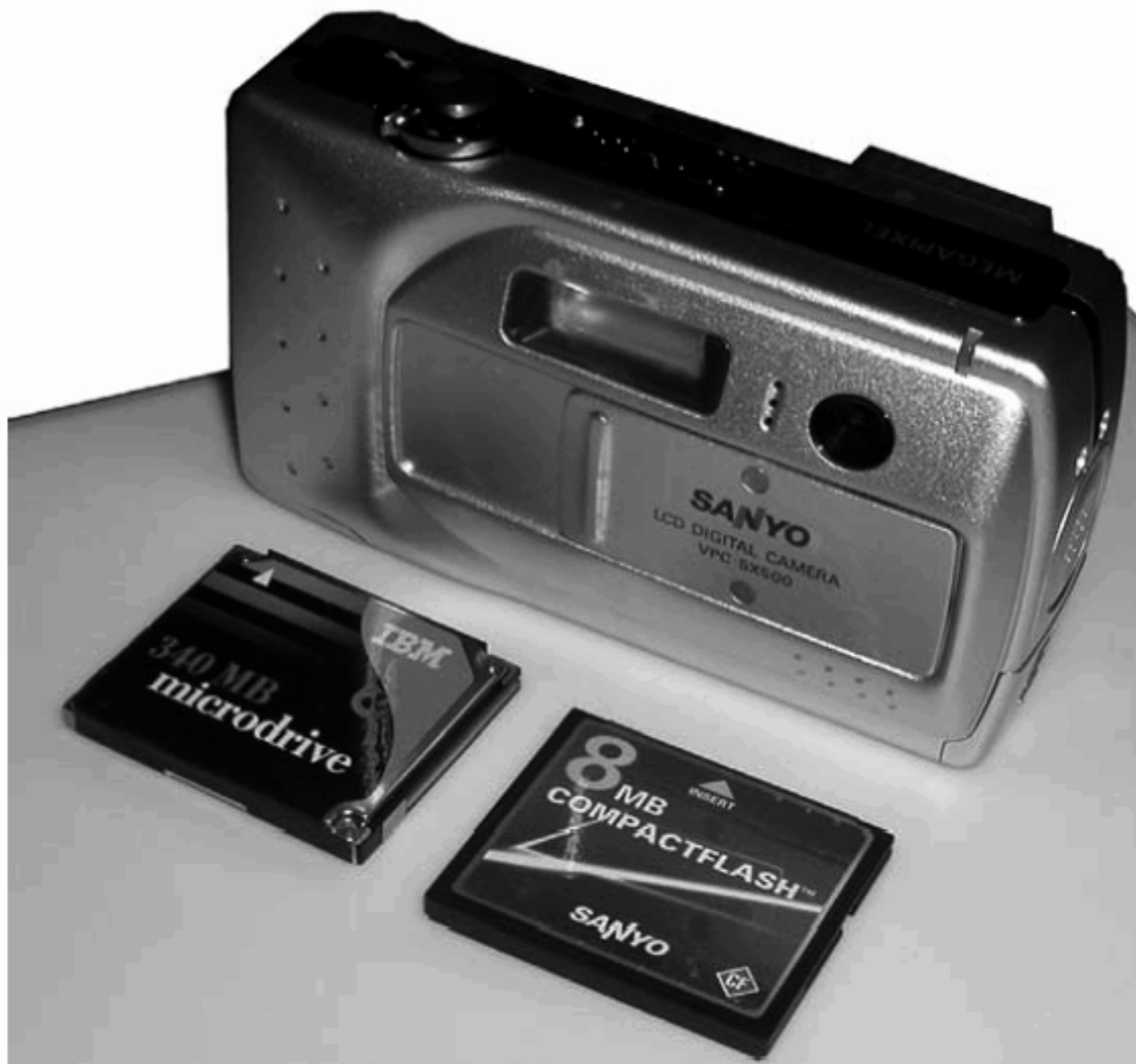
FIGURE 8.14 The Sanyo VPC-SX500 with Flash memory card and IBM Microdrive. Although newer cameras offer more pixels per picture, the principles are the same. This 1360 \times 1024 pixel digital camera stores pictures either using CompactFlash memory or using a IBM Microdrive. This photo was taken using a 340 MB microdrive and a 8 MB CompactFlash memory. As Figure 8.15 shows, in 2004 the capacities are as large as 1 GB to 4 GB. It is 4.3 inches wide \times 2.5 inches high \times 1.6 inches deep, and it weighs 7.4 ounces. In addition to taking a still picture and converting it to JPEG format every 0.9 seconds, it can record a Quick Time video clip at VGA size ( 640 \times 480 ). One technological advantage is the use of a custom system on a chip to reduce size and power, so the camera only needs two AA batteries to operate versus four in other digital cameras.
