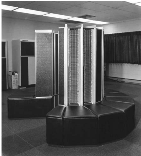
FIGURE e1.13.4 Cray-1, the first commercial vector supercomputer, announced in 1976. This machine had the unusual distinction of being both the fastest computer for scientific applications and the computer with the best price/performance for those applications. Viewed from the top, the computer looks like the letter C. Seymour Cray passed away in 1996 because of injuries sustained in an automobile accident. At the time of his death, this 70-year-old computer pioneer was working on his vision of the next generation of supercomputers. (See www.cray.com for more details.)
