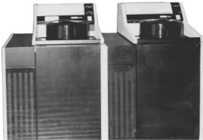
FIGURE e5.17.7 This is a DEC disk drive and the removable pack. These disks became popular starting in the mid-1960s and dominated disk technology until Winchester drives in the late 1970s. This drive was made in the mid-1970s; each disk pack in this drive could hold 80 MB.
