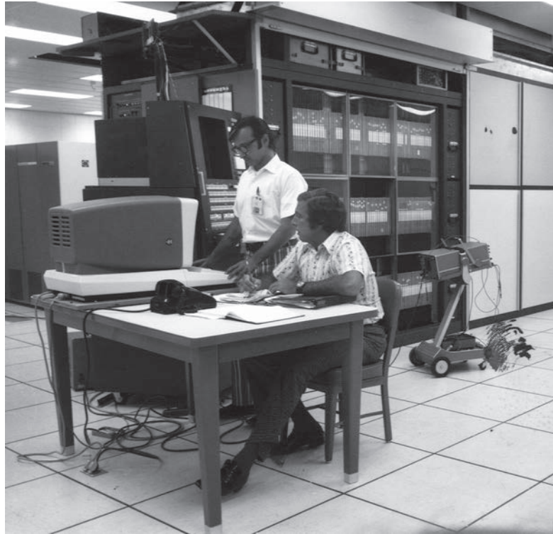
FIGURE e6.16.1 The Illiac IV control unit followed by its 64 processing elements. It was perhaps the most infamous of supercomputers. The project started in 1965 and ran its first real application in 1976. The 64 processors used a 13-MHz clock, and their combined main memory size was 1 MB: 64 \times 16 KB. The Illiac IV was the first machine to teach us that software for parallel machines dominates hardware issues. Photo courtesy of NASA Ames Research Center.
