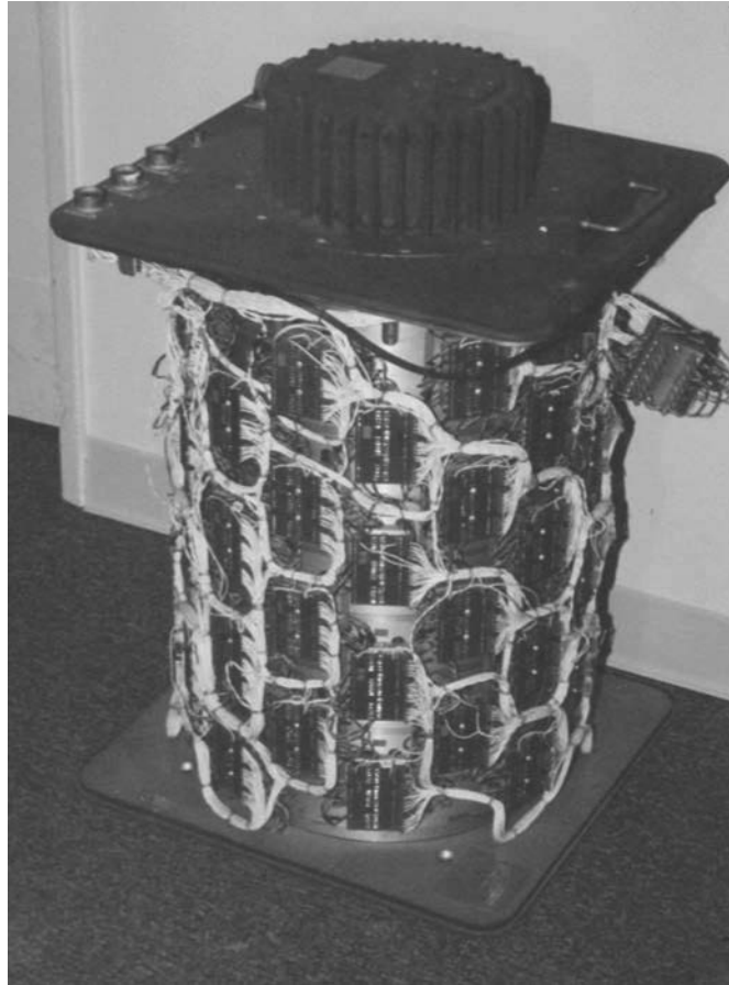
FIGURE e5.17.5 A magnetic drum made by Digital Development Corporation in the 1960s and used on a CDC machine. The electronics supporting the read/write heads can be seen on the outside of the drum.
