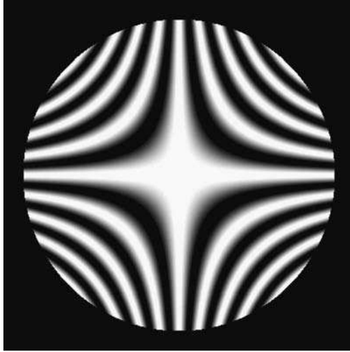
FIGURE 5.25. Astigmatism pattern in a rotational shear interferometer with maximum sensitivity ( \phi = 90^\circ )( \alpha_{22} = 2\lambda ).
