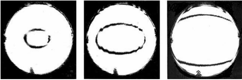
FIGURE 8.28. Shadow patterns obtained when using a \lambda/2 phase edge for testing a lens with comatic aberrations.
