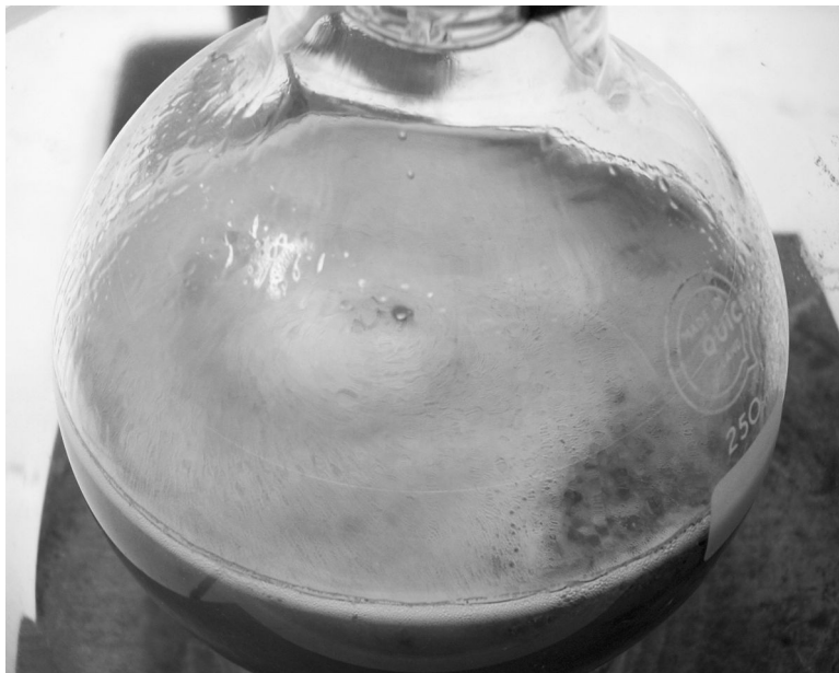
FIGURE 9.2 In this in situ preparation of \text{LiAlH}_4 , \text{Al}_2\text{Br}_6 solution is slowly added to \text{LiH} , maintaining a gentle ether reflux using the moderate exothermicity of this acid/base reaction. Large grains of \text{LiH} react and dissolve in about 20 min, forming a \text{LiAlH}_4 solution, which is extremely sensitive to minute traces of moisture. Decomposition occurs over several days, depositing large grains of polymeric \text{AlH}_3 .
