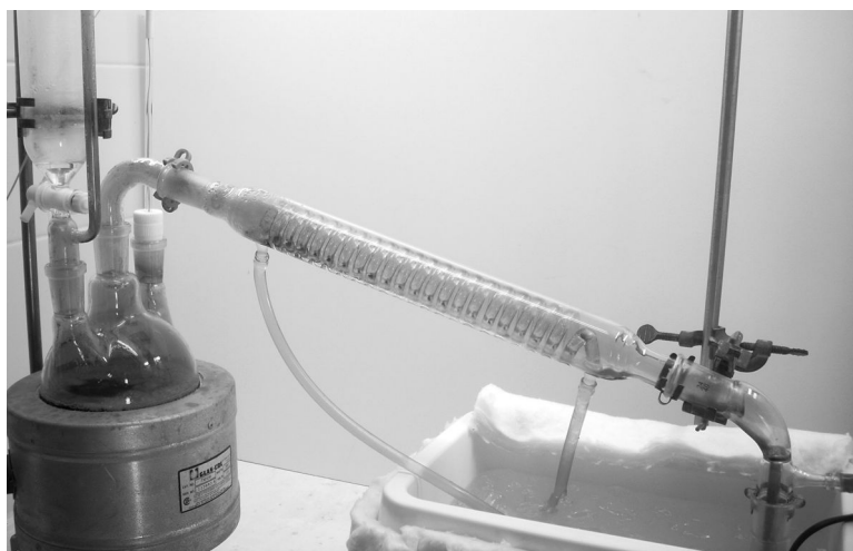
FIGURE 7.1 Sodium sulfite solution at room temperature instantaneously reduces BCDMH generating bromine.
