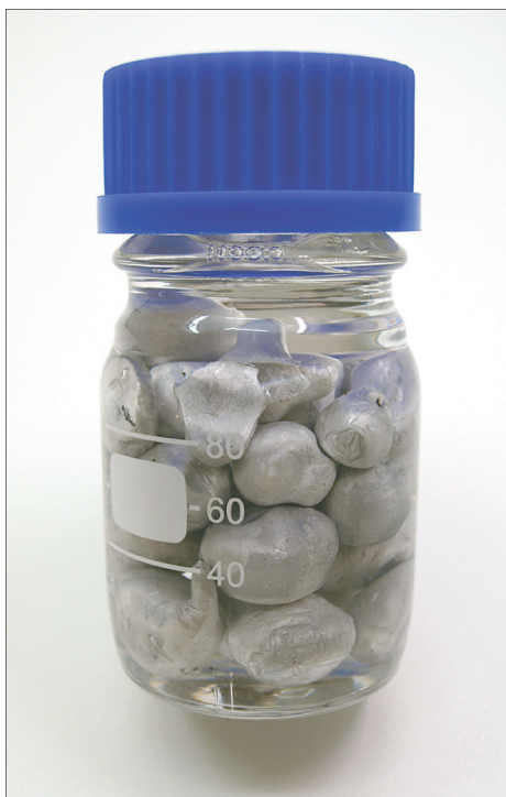
FIGURE 2.6 Sodium as it is collected from the cell and stored beneath liquid paraffin.
