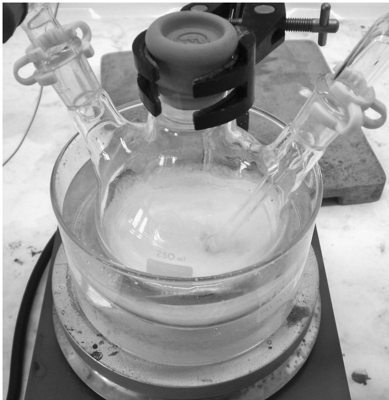
FIGURE 13.2 A color version of this figure follows page 112. Schlosser's base at -10^{\circ}\text{C} metallates gaseous hydrogen with the formation of a white potassium hydride precipitate. The hydride is stable at room temperature; however, being pyrophoric in air, it is used in situ.
