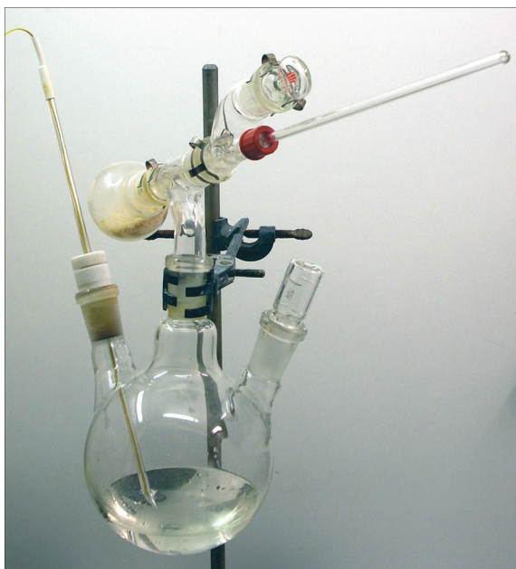
FIGURE 9.1 Aluminum bromide, which decomposes many organic solvents, is here slowly added to diethyl ether with the temperature maintained below 0°C by rapid swirling and cooling the ether in a freezing mixture. The glass stopper is replaced by a \text{CaCl}_2 protection tube prior to dissolution.
