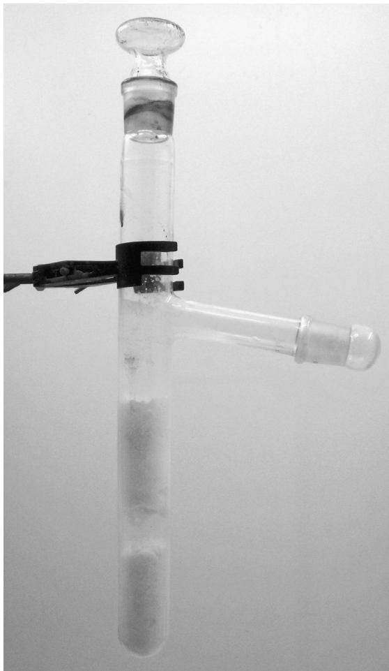
FIGURE 20.3 Quartz test tube with distillation side arm containing the \text{Na}_2\text{SO}_4 product at the end of the experiment.
