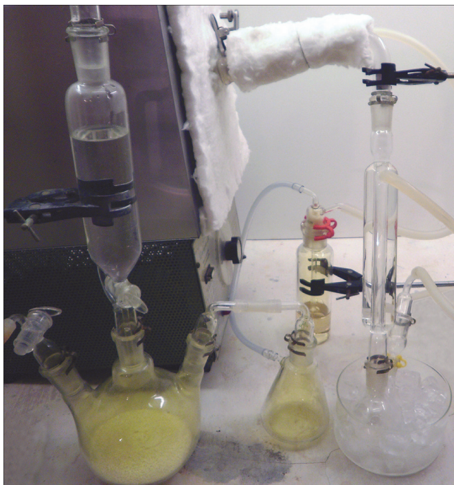
FIGURE 19.1 A mixture of powdered carbon and \text{Ca}_3(\text{PO}_4)_2 is chlorinated at 760^\circ\text{C} . Initially, \text{Ca}_3(\text{PO}_4)_2 is converted to \text{Ca}(\text{PO}_3)_2 . Subsequently, \text{POCl}_3 forms and collects in the receiver. The gaseous products include \text{CO} and \text{COCl}_2 ; hence, the preparation is conducted inside a fume hood.
