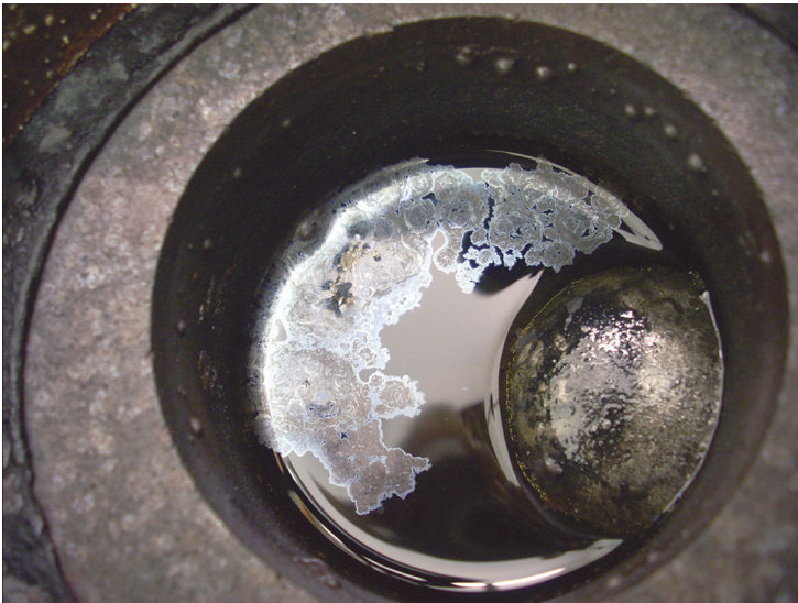
FIGURE 4.1 A lithium globule on the surface of a molten KCl–LiCl eutectic at 420°C after electrolysis. At this temperature, lithium ordinarily burns in air; however, a thin film of electrolyte protects it. The film is made visible by traces of carbon from the anode adhering to the surface.
