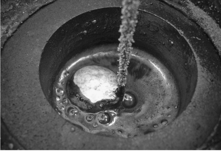
FIGURE 4.3 A color version of this figure follows page 112. The molten lithium acts as the cathode being attracted to the steel electrode by electrical forces. This arrangement uses the surface tension of lithium to reduce its fragmentation, which otherwise leads to small lithium globules reaching the anode where their protective electrolyte coat is broken and an explosive reaction with chlorine results.
