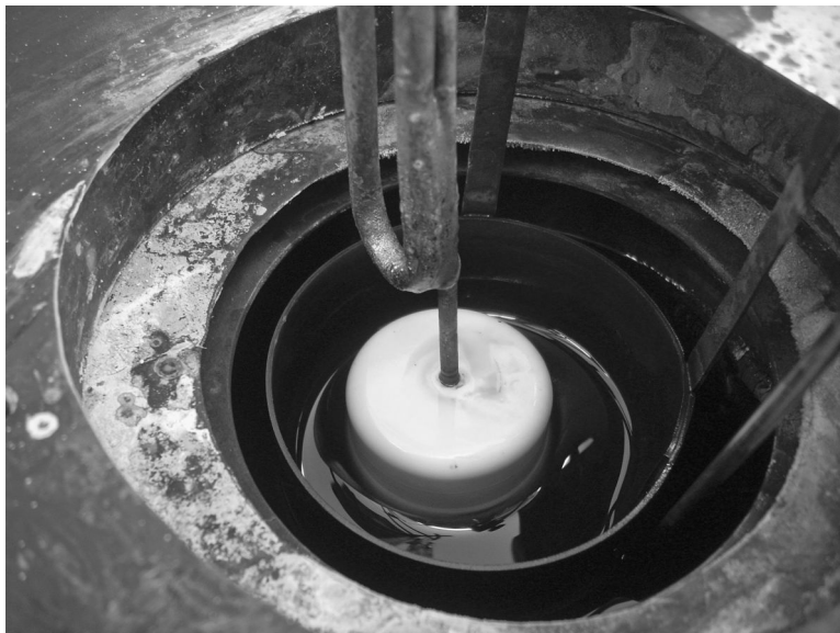
FIGURE 3.2 A color version of this figure follows page 112. A 3-in.-long MgO crucible, which is not attacked by the caustic, is used to separate the anode and cathode compartments in the KOH cell. A water-cooled copper tube acts as the cathode and supports the crucible. Unlike the NaOH case, no hydrogen is generated in the cathode compartment; however, the copper–MgO juncture is not airtight to allow the fluid level inside the crucible to equilibrate.
