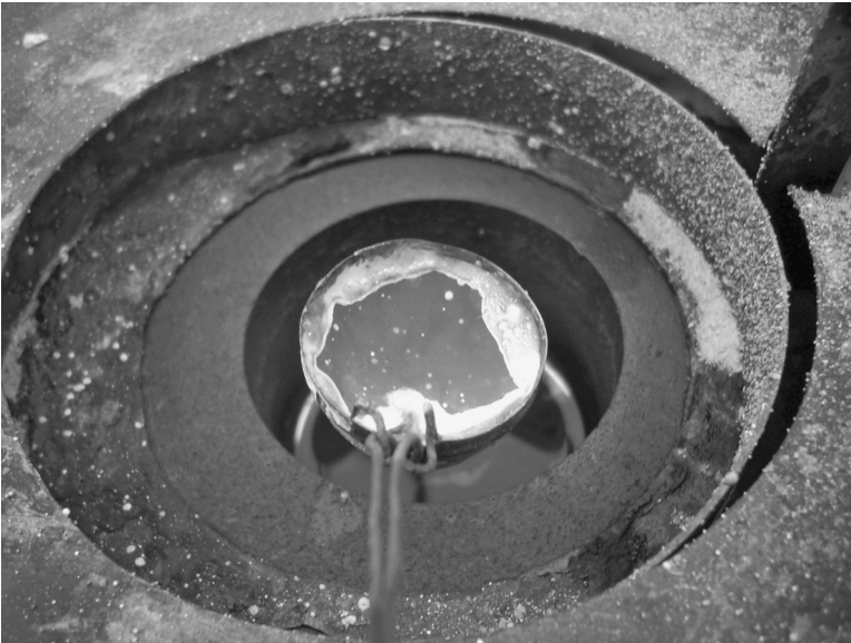
FIGURE 4.4 A color version of this figure follows page 112. Lithium is collected from the cell with a perforated ladle. With the protective coat of electrolyte broken, surface oxidation commences and the molten lithium may ignite. It is thus quickly run into paraffin and held down with steel gauze.
