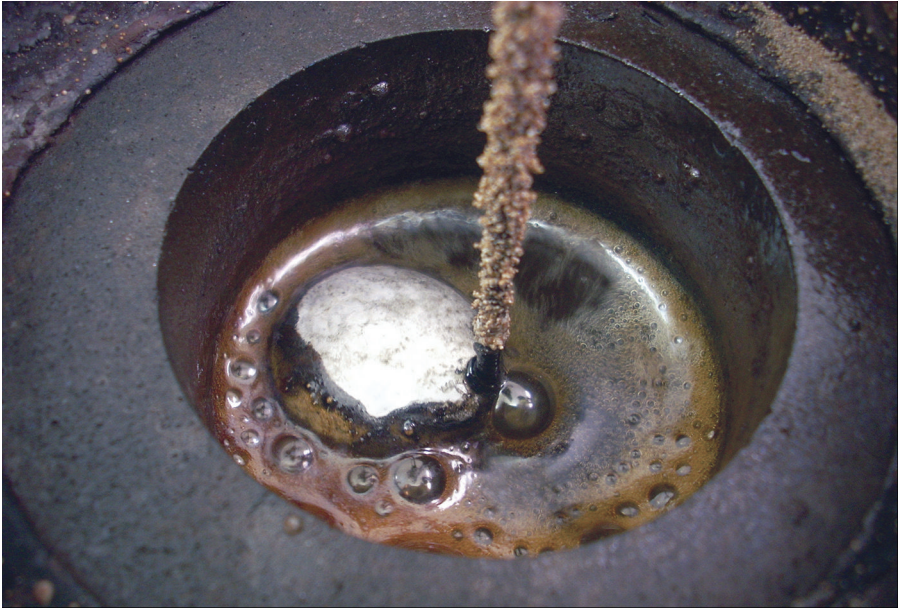
FIGURE 4.3 The molten lithium acts as the cathode being attracted to the steel electrode by electrical forces. This arrangement uses the surface tension of lithium to reduce its fragmentation, which otherwise leads to small lithium globules reaching the anode where their protective electrolyte coat is broken and an explosive reaction with chlorine results.
