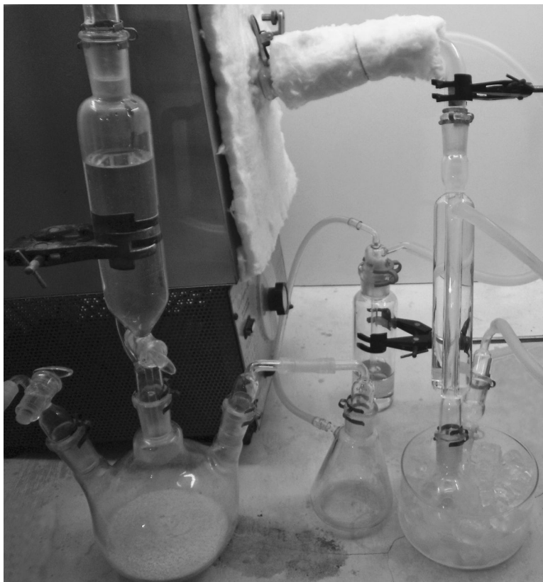
FIGURE 19.1 A color version of this figure follows page 112. A mixture of powdered carbon and \text{Ca}_3(\text{PO}_4)_2 is chlorinated at 760^\circ\text{C} . Initially, \text{Ca}_3(\text{PO}_4)_2 is converted to \text{Ca}(\text{PO}_3)_2 . Subsequently, \text{POCl}_3 forms and collects in the receiver. The gaseous products include \text{CO} and \text{COCl}_2 ; hence, the preparation is conducted inside a fume hood.
