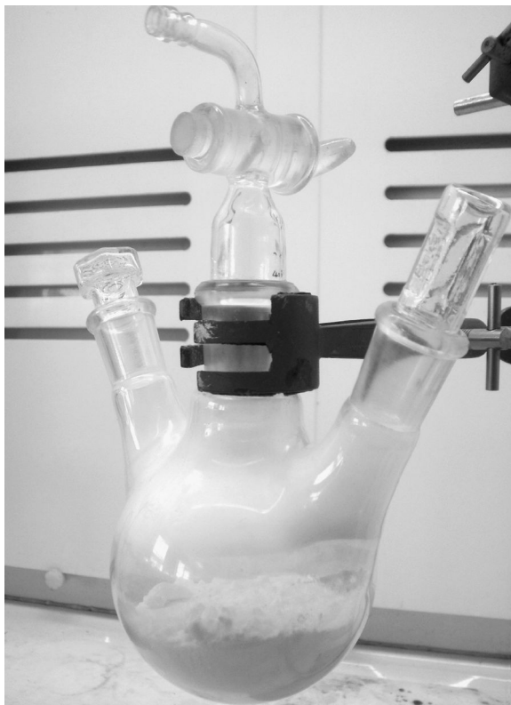
FIGURE 13.1 Potassium t -butoxide, formed by the reaction of potassium metal with excess t -butanol, exists in the solid state as clusters held together by weak bridge bonds. It, therefore, sublimates at relatively low temperatures and separation from the parent alcohol, which is needed to increase its pH, must be performed under carefully controlled conditions.
