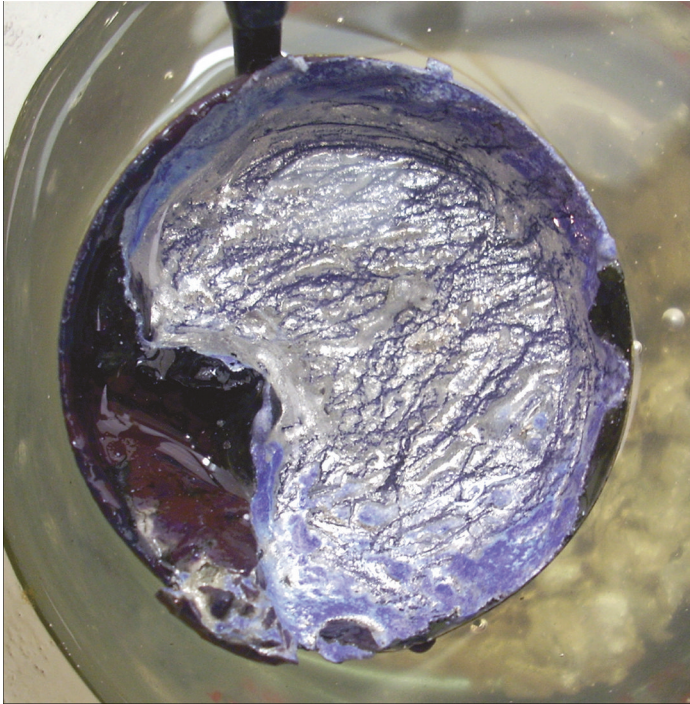
FIGURE 3.3 When the contents of the metal ladle have cooled under paraffin, the potassium is scraped from the solidified KOH layer below into the paraffin-filled container. The potassium has a blue-violet tinge due to traces of oxygen, and resembles soft butter in consistency.
