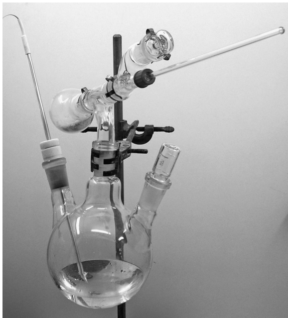
FIGURE 9.1 A color version of this figure follows page 112. Aluminum bromide, which decomposes many organic solvents, is here slowly added to diethyl ether with the temperature maintained below 0^{\circ}\text{C} by rapid swirling and cooling the ether in a freezing mixture. The glass stopper is replaced by a \text{CaCl}_2 protection tube prior to dissolution.
