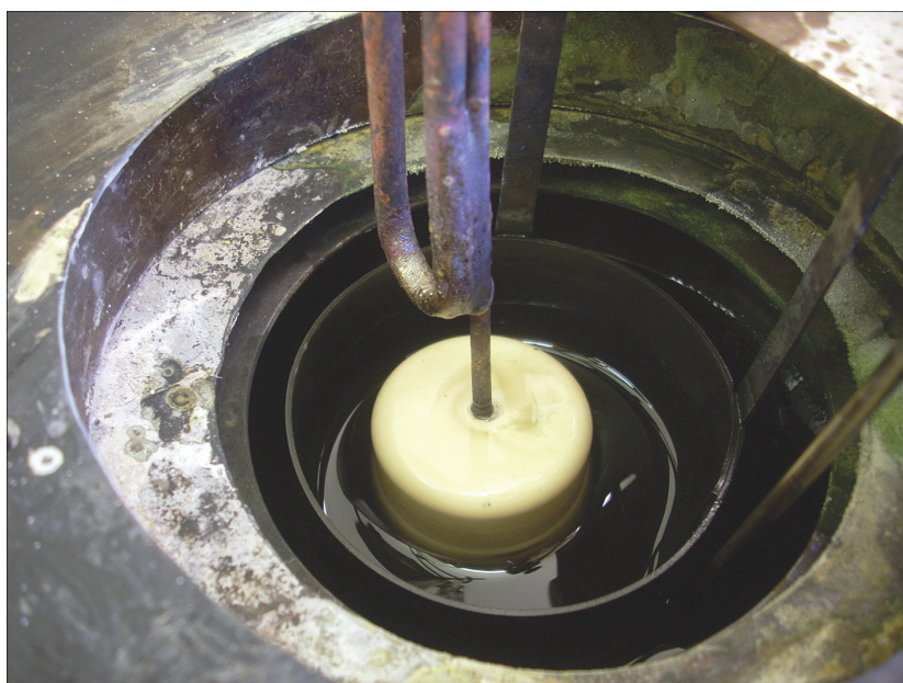
FIGURE 3.2 A 3-in.-long MgO crucible, which is not attacked by the caustic, is used to separate the anode and cathode compartments in the KOH cell. A water-cooled copper tube acts as the cathode and supports the crucible. Unlike the NaOH case, no hydrogen is generated in the cathode compartment; however, the copper–MgO juncture is not airtight to allow the fluid level inside the crucible to equilibrate.
