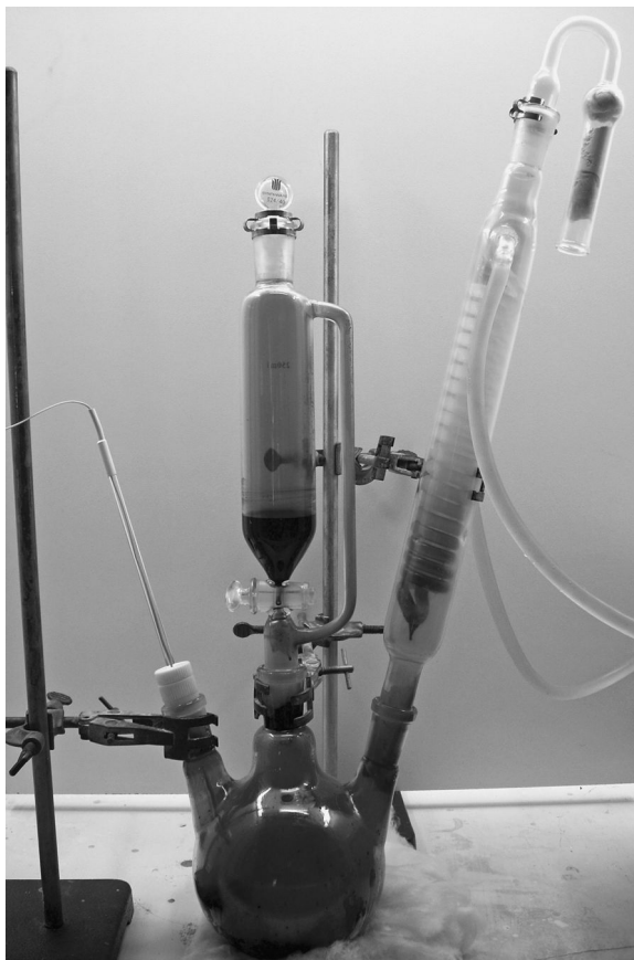
FIGURE 8.1 A color version of this figure follows page 112. Bromine reacts with aluminum granules accompanied by sporadic flashing with the temperature rising to 210°C–220°C. The heat volatilizes the unreacted bromine, which refluxes in the condenser until it is all consumed. On cooling, the \text{Al}_2\text{Br}_6 product crystallizes as white scaly crystals on the flask walls.
