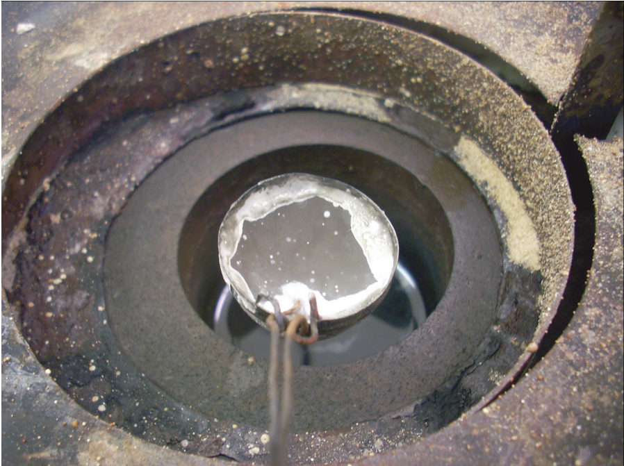
FIGURE 4.4 Lithium is collected from the cell with a perforated ladle. With the protective coat of electrolyte broken, surface oxidation commences and the molten lithium may ignite. It is thus quickly run into paraffin and held down with steel gauze.
