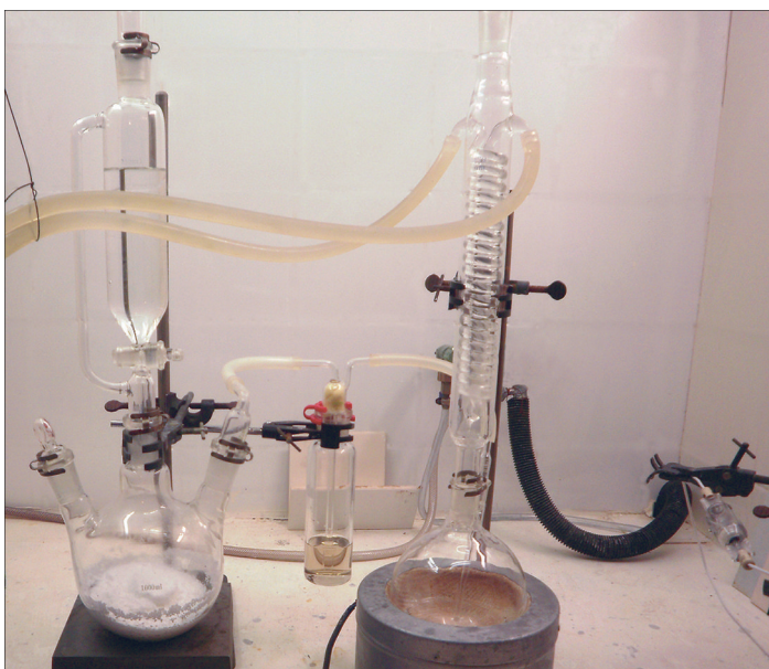
FIGURE 16.4 Experimental setup for photolytic chlorination of chloroform. The chlorine generator, described in Chapter 15, is on the left in the photo. The 1-kW, high-pressure, mercury vapor lamp is on the right.
