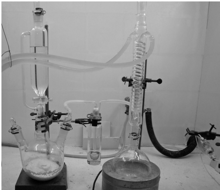
FIGURE 16.4 A color version of this figure follows page 112. Experimental setup for photolytic chlorination of chloroform. The chlorine generator, described in Chapter 15, is on the left in the photo. The 1-kW, high-pressure, mercury vapor lamp is on the right in the photo.
