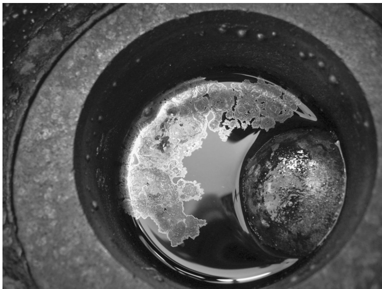
FIGURE 4.1 A color version of this figure follows page 112. A lithium globule on the surface of a molten KCl–LiCl eutectic at 420^\circ\text{C} after electrolysis. At this temperature, lithium ordinarily burns in air; however, a thin film of electrolyte protects it. The film is made visible by traces of carbon from the anode adhering to the surface.
