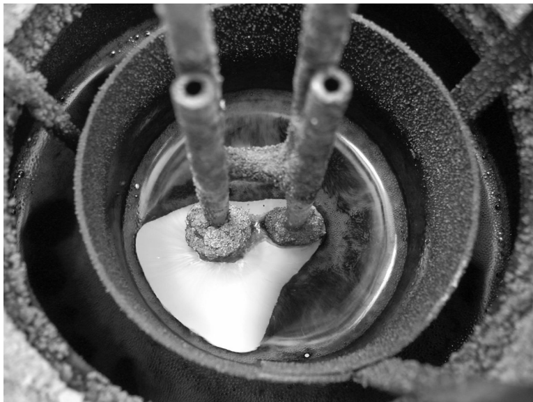
FIGURE 2.5 A color version of this figure follows page 112. The nickel separator dipping below the molten NaOH encloses the cathode and forms the acid/base interface in the cell, and the region where hydrogen is generated. In Regime 2, this prevents sodium from shorting the separator to the cathode. The cathode consists of liquid sodium attracted by electrical forces to a water-cooled copper electrode raised just above the surface of the melt.
