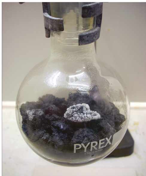
FIGURE 10.2 The reaction between sodium and \text{Et}_2\text{BrAl} commences at the melting point of sodium and becomes extremely vigorous at about 107^\circ\text{C} . After a few minutes, the flask fills with large, black, porous pieces of Al-NaBr aggregate that soak up the \text{Et}_3\text{Al} product.
