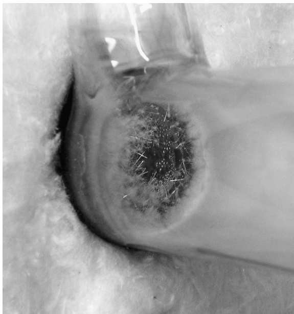
FIGURE 6.2 A color version of this figure follows page 112. Sodium evaporating from an oven at 600°C, in hydrogen at 1 atm. NaH needles form in a section of the reactor where the temperature is such that hydrogen pressure above NaH is below 1 atm.
