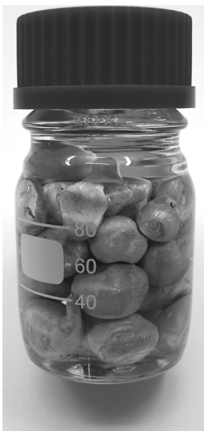
FIGURE 2.6 A color version of this figure follows page 112. Sodium as it is collected from the cell and stored beneath liquid paraffin.
