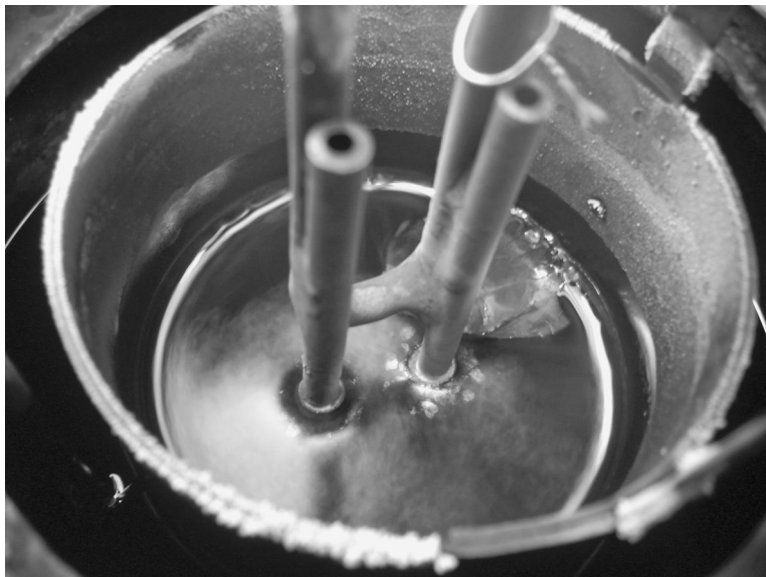
FIGURE 3.1 A color version of this figure follows page 112. Molten KOH at 410°C electrolyzed in the same arrangement as NaOH with currents in the range 10–50 A, produces fleeting metallic streaks in the vicinity of the cathode. Fuming is greatly decreased under a protective argon stream, but no potassium globules are formed, nor is oxygen effervescence observed at the anode.
