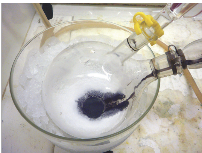
FIGURE 20.4 The fraction above 500^\circ\text{C} from \text{NaHSO}_4 pyrolysis. Liquid oleum, colored black from carbonization of silicon grease, collects in the receiver below 580^\circ\text{C} ; above this temperature, nearly pure \text{SO}_3 deposits on the chilled flask walls by sublimation from the reactor.
