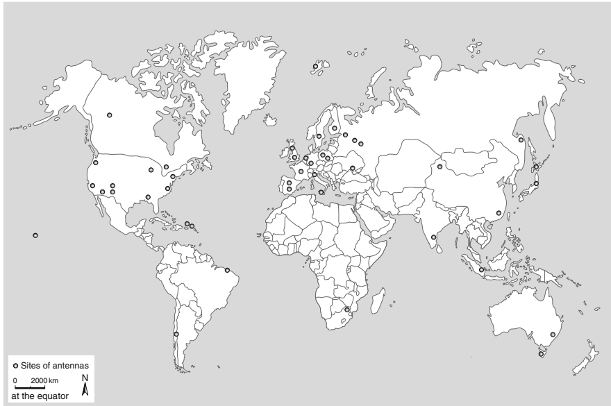
Fig. 6.42 Worldwide network of radiotelescopes which can be combined in VLBI observations (2007). Regional networks are organised in Europe with the European VLBI Network (EVN), and in the USA with the Very Long Baseline Array (VLBA). Most of the instruments featured here are radiotelescopes, but some are specific to terrestrial geodesy, using VLBI to study continental drift and the deformations of the land masses over time. New instruments are frequently added to this network, e.g., the Antarctic
