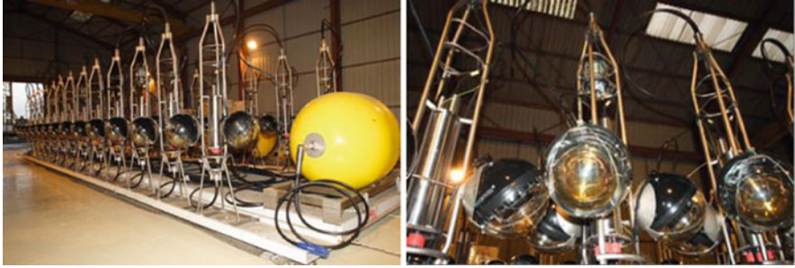
Fig. 7.61 Left: Photograph of a detection string in the assembly room, folded up on a pallet, just prior to immersion. Right: Photograph of one storey of a detector string, showing the photodetectors inside their protective spheres. The associated electronics is housed in a central titanium container
