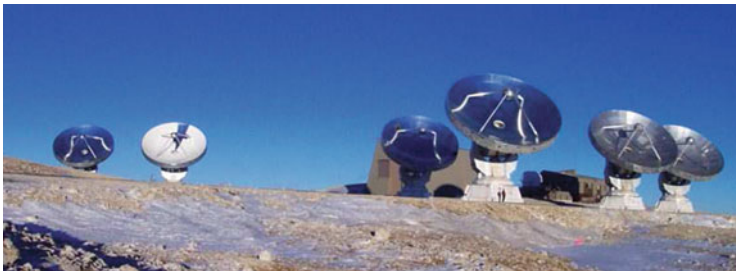
Fig. 6.38 The radio interferometer at the Plateau de Bure (France), operating at millimetre wavelengths
