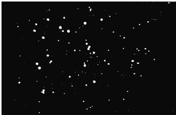
Fig. 7.24 Photon counts, as they appear on the TV screen of a Nocticon tube (exposure 25 ms). Note the variable gain, manifested by the varying brightness of the events. Note also the noise events, fainter and easy to discriminate. The image is read on a 512 \times 512 CCD array. Each event is digitally centered. (Observatoire de Marseille, image due to Boulesteix J. in the 1980s)
