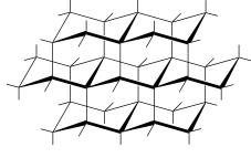
**FIGURE 4.27** The structure of diamonds.
