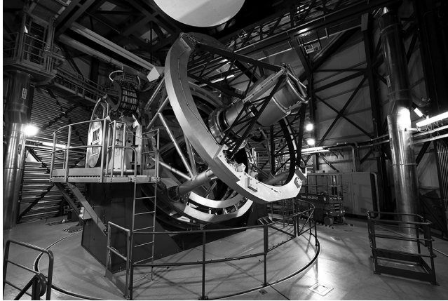
FIGURE 1.21 European Southern Observatory’s (ESO’s) 4.1-m Visible and Infrared Survey Telescope for Astronomy (VISTA) telescope. The large metal cylinder mounted at and projecting beyond the top ring of the telescope is the infrared camera containing the cryostat, baffles, filters, and of course, the 67.1-megapixel detector array. (Courtesy of ESO.)
