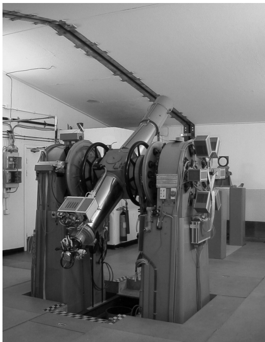
FIGURE 5.4 A transit telescope – the Carlsberg Meridian Telescope on La Palma. Decommissioned 2013. (Courtesy of D. W. Evans.)
