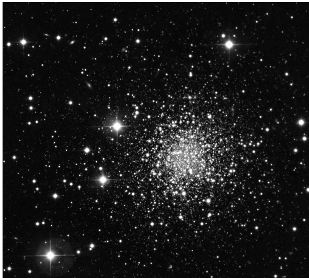
FIGURE 1.34 Diffraction spikes on images of bright stars arising from the secondary mirror supports. (Detail from an image of the globular cluster NGC 2257 obtained with the Wide Field Imager instrument on the 2.2-m Max Planck Gesellschaft/European Southern Observatory (MPG/ESO) telescope at La Silla. (Courtesy of ESO.)
