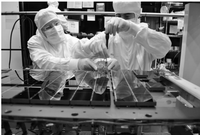
FIGURE 1.13 Part of the Gaia charge-coupled device (CCD) mosaic during its assembly. (Courtesy of Astrium.)
