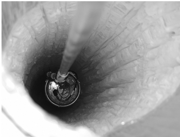
FIGURE 1.107 Top, One of the pressure spheres containing the photomultiplier and electronics for the IceCube neutrino telescope ready to be lowered into position. (Courtesy of IceCube Collaboration/National Science Foundation [NSF]). Bottom, The IceCube pressure sphere on its way down through the hole drilled into the Antarctic icecap. (Courtesy of IceCube Collaboration/NSF.)
