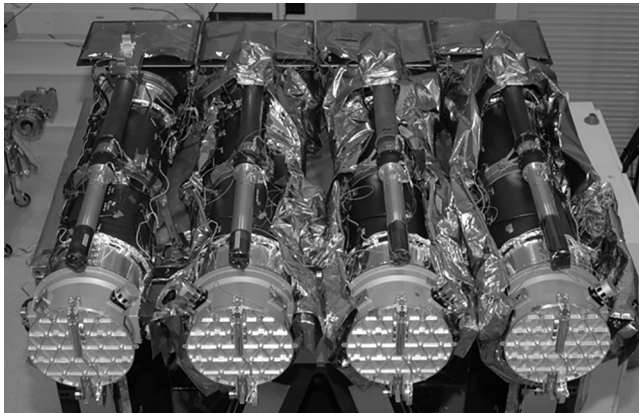
FIGURE 1.24 The Atmospheric Imaging Assembly (AIA) instrument for the Solar Dynamic Observatory (SDO) spacecraft during its assembly. The image shows the four 0.2-m telescopes with their protective front covers in place. The charge-coupled device (CCD) array detectors are at the far ends of the telescopes. (Courtesy of National Aeronautics and Space Administration [NASA].)
