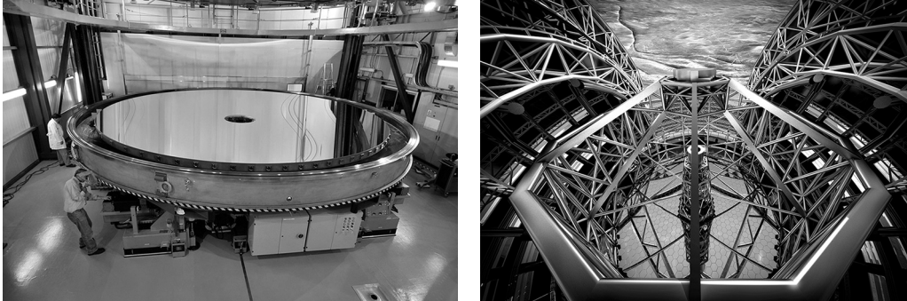
FIGURE 1.30 Left, The 8.2-m monolithic primary mirror of 'Yepun' (Mapuche language word for the Evening Star, Venus) – one of the four main instruments comprising European Southern Observatory's (ESO's) Very Large Telescope (VLT). (Courtesy of ESO/G. Huedepohl). Right, An artist's concept of the 39.3-m main mirror of the future Extremely Large Telescope (ELT) clearly showing the hexagonal segments from which it is made. (Courtesy of ESO/L. Calçada/Ace Consortium.)
