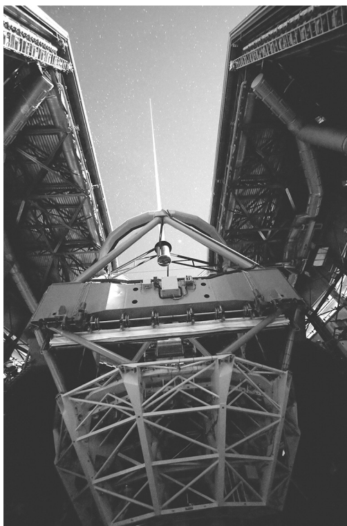
FIGURE 1.64 A single laser beam being sent from the Very Large Telescope's (VLT)'s Yepun telescope to produce an artificial guide star. See also Figure 1.68 . (Courtesy of European Southern Observatory/Y. Beletsky.)
