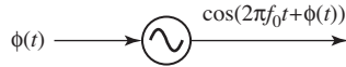
Figure 3.4 An oscillator creates a sinusoidal oscillation with a specified frequency f_0 and input \phi(t) .
