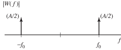
Figure 4.9 The magnitude spectrum of a sinusoid with frequency f_0 and amplitude A contains two \delta -function spikes, one at f = f_0 and the other at f = -f_0 .
