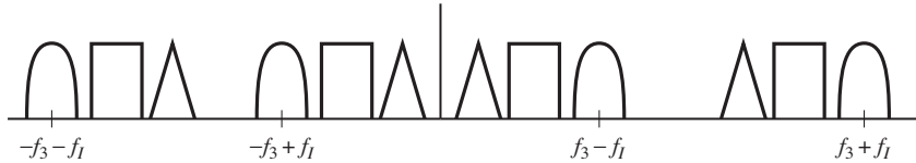
Figure 2.9 FDM downconversion to an intermediate frequency.
