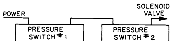
Fig. B-2 Noncomplex series redundancy. This type of redundancy guards against inadvertent closing; i.e., closing when not called upon to close.
