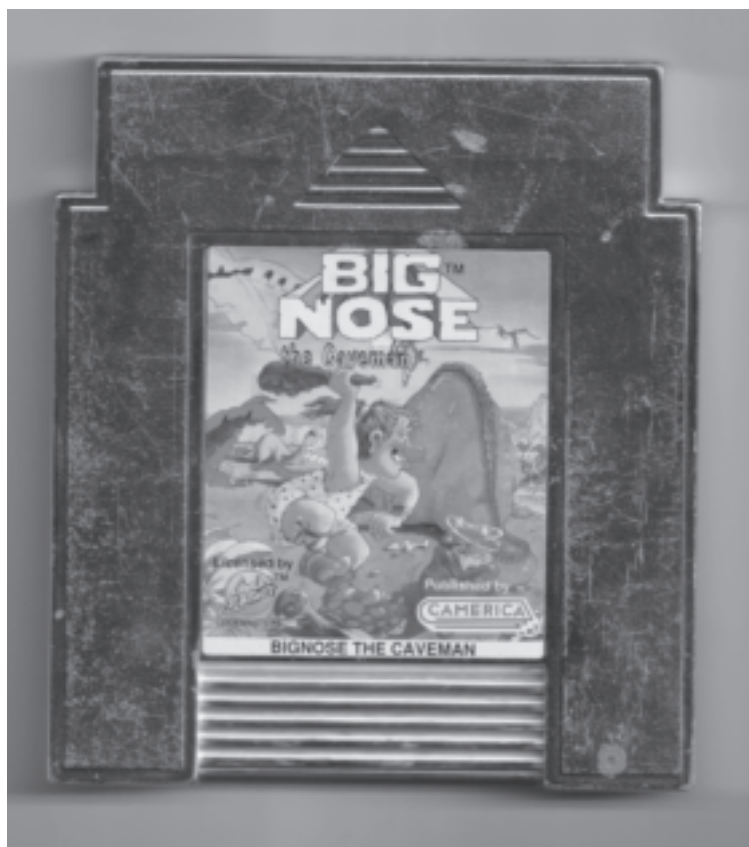
Figure 25.2: Unlicensed Cartridge without a CIC
