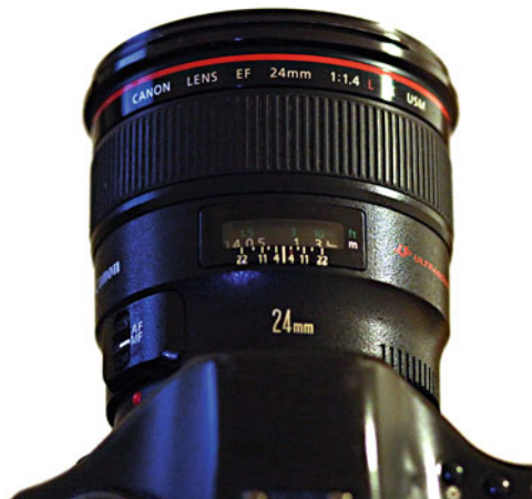
Fig. 6 A fast 24 mm lens with a widest aperture of 1.4 is an ideal standard lens of nightscape photography
