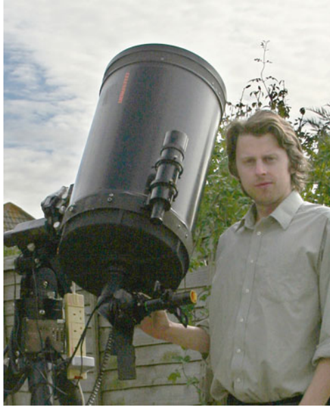
Fig. 2 My own primary telescope – a Celestron 36 cm SCT on a German equatorial mount (Photo by the author)
