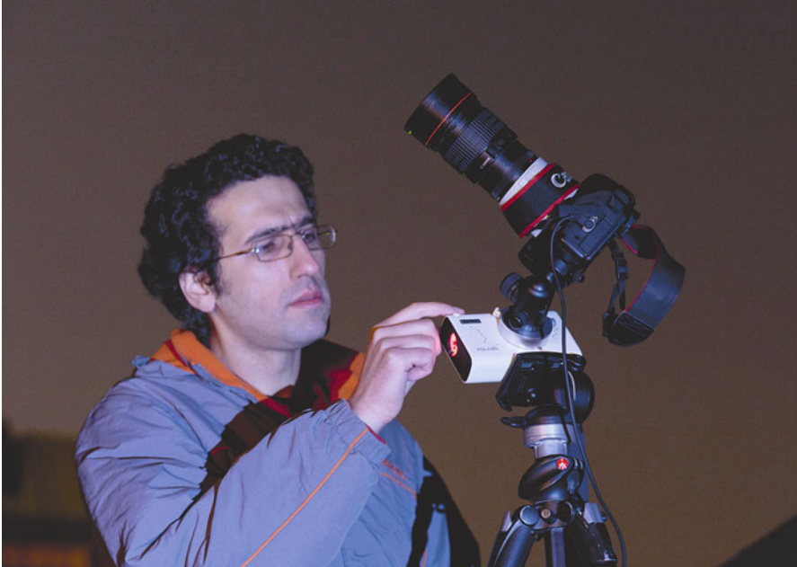
Fig. 12 A portable star tracking mount such as Polarie is a very helpful accessory to reach more sky details in landscape astrophotography
