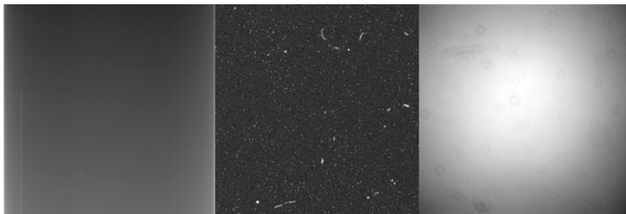
Fig. 2 Left: stretched bias file. Middle: crop of stretched dark file 15 min. Right: stretched flat field file
