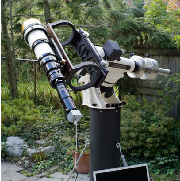
Fig. 4 The author's main solar telescope for imaging at the hydrogen alpha wavelength – a 92 mm f4.8 Astro-Physics refractor with a 90 mm .7 \text{ \AA} Coronado Ha filter. A Barlow and a streaming camera from Point Grey Research are attached at the focuser end
