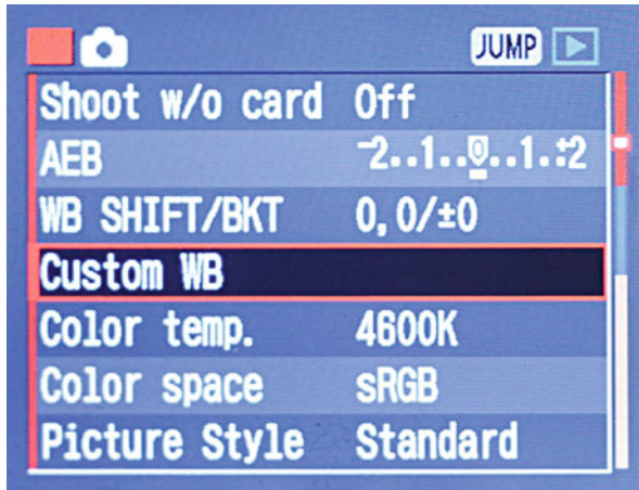
Fig. 23 While adjusting the white balance is possible in the post processing (using RAW files) you can also precisely set this in the camera using the custom white balance function, similar to white balancing video cameras
