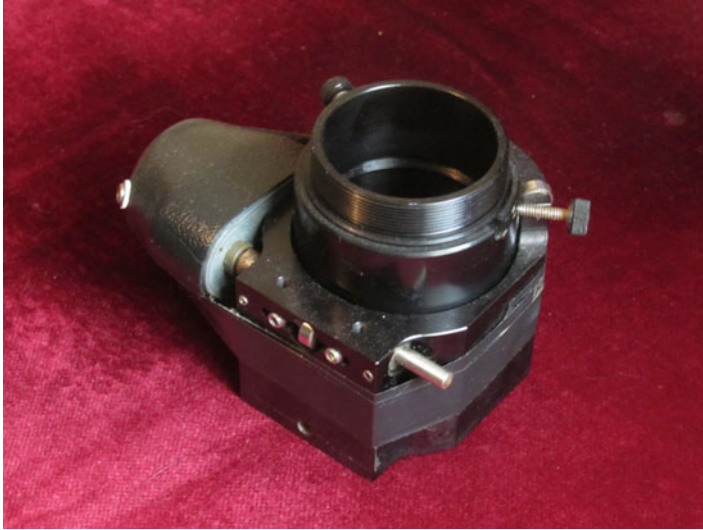
Fig. 7 A motorized focuser that allows focusing without having to touch the telescope is an essential piece of equipment for planetary imaging. This JMI unit pictured is a popular choice among observers (Photo by the author)
