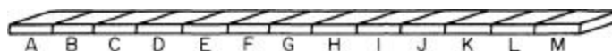
FIGURE 21. To calculate more easily where the light goes, we shall temporarily consider only a strip of mirror divided into little squares, with one path for each square. This simplification in no way detracts from an accurate analysis of the situation.
