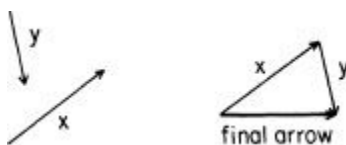
FIGURE 8. Arrows that represent each possible way an event could happen are drawn and then combined ("added") in the following manner: Attach the head of one arrow to the tail of another—without changing the direction of either one—and draw a "final arrow" from the tail of the first arrow to the head of the last one.
