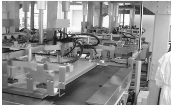
FIGURE 6.12 Automated build-up of copper and prepreg.
