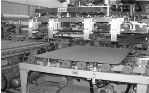
FIGURE 6.11 Automated build-up of copper and prepreg.
