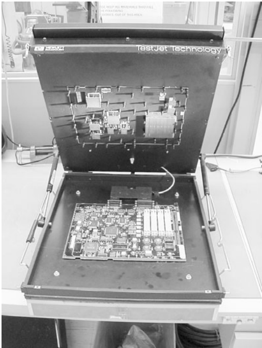
FIGURE 55.14 A test fixture with board on a bed of nails, with clamshell top fixture containing capacitive sensor plates. Notice eight closely spaced sensor plates (right) that test for opens in eight (white) connectors on the board.
