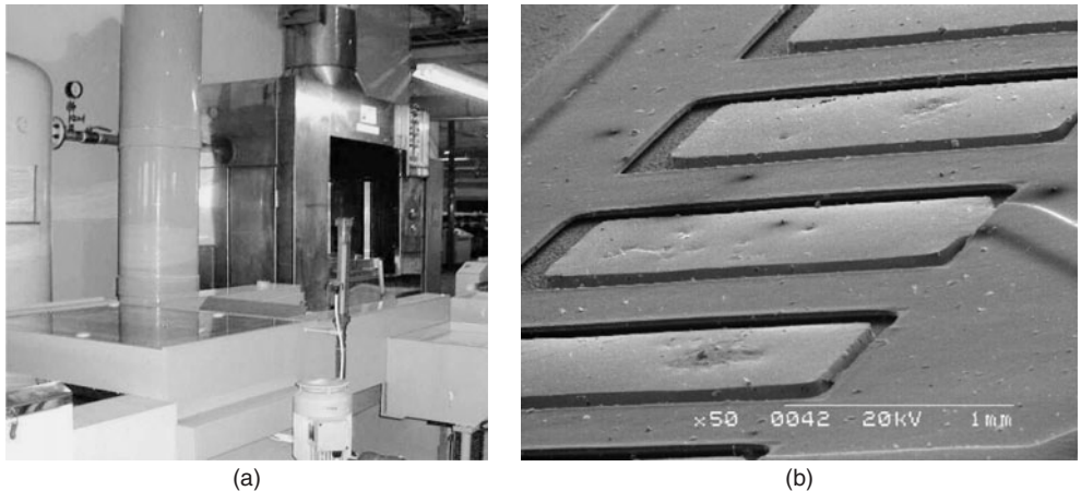
FIGURE 32.2 (a) HASL equipment (b) surface scanning electron micrograph (SEM).
