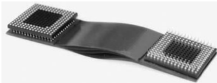
FIGURE 65.2 Air gap structure of multilayer rigid-flex board.
