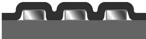
FIGURE 51.11 Soda straws between copper trace and soldermask. (courtesy of IPC.)
