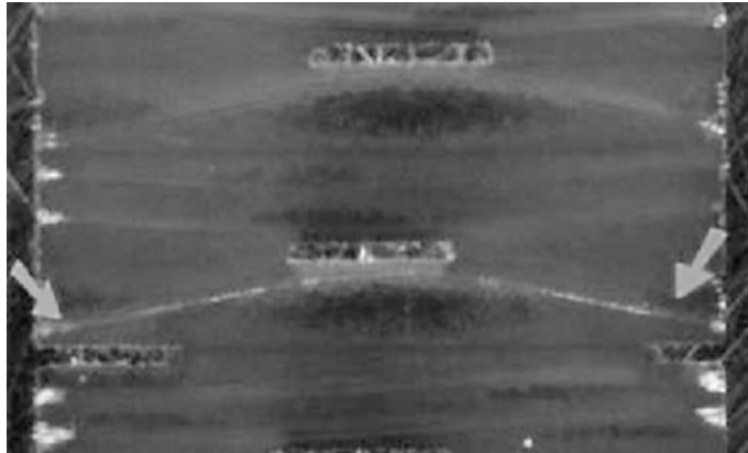
FIGURE 9.13 An example of CAF between two plated through holes.
