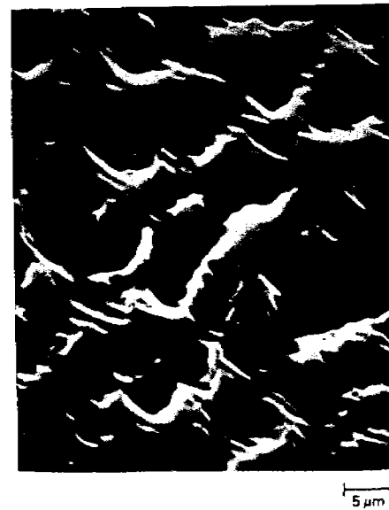
Figure 7.13 Speckle pattern obtained from exposing a pattern using a narrow linewidth laser as the optical source (after Jain).
