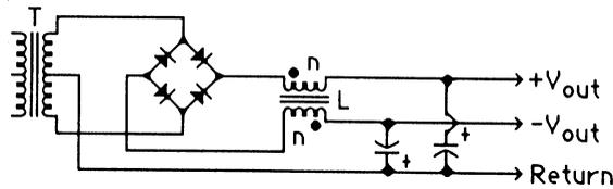
Figure 3-21 The mutually coupled output filter choke.
