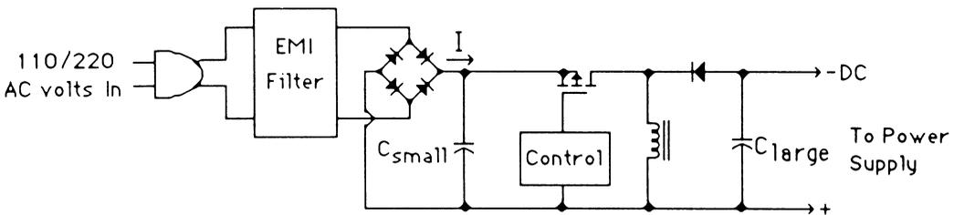
Figure C-4 A buck/boost power factor correction circuit.
