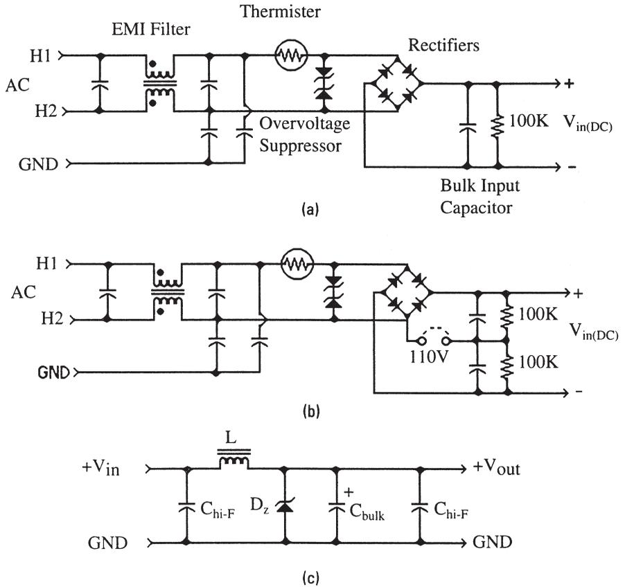
**Figure 3-54** Typical ac and dc input filter circuits: (a) ac input filter circuit for a single or universal input power supply (common-mode EMI filter shown); (b) a voltage doubling ac input circuit for 110 V and 220 V ac inputs; (c) single dc bus input filter.
