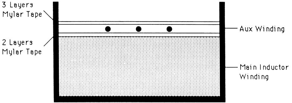
Figure C-8 Construction of the PFC boost inductor.
