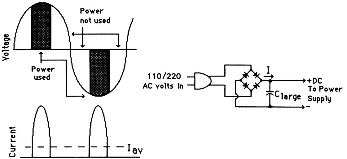
Figure C-1 The waveforms of a capacitive input filter.
