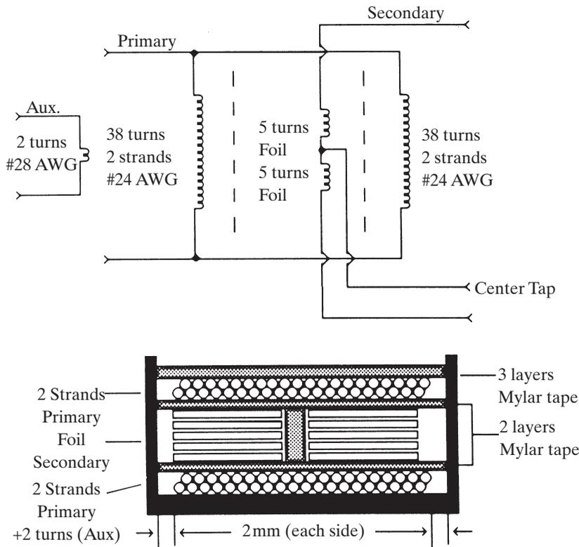
**Figure 3-73** Transformer construction.
