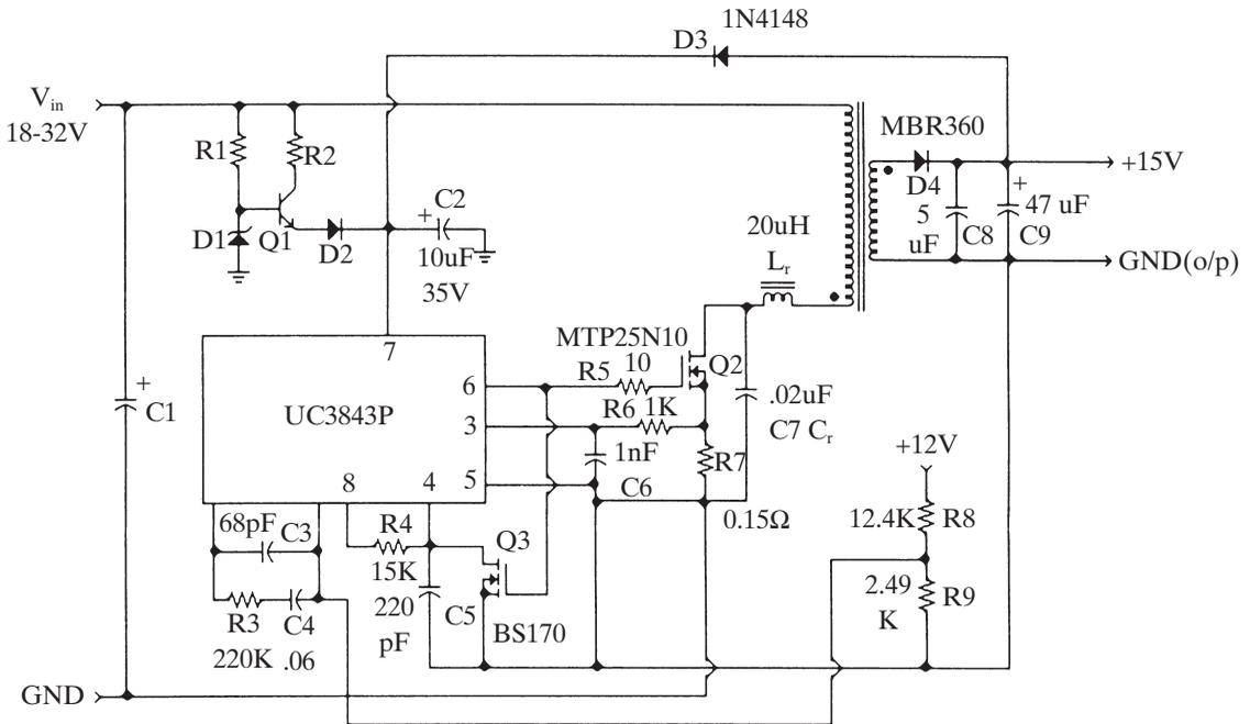
Figure 4-22 A ZVS quasi-resonant current-mode flyback converter.
