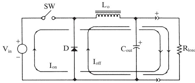
Figure 3-1 A basic forward-mode converter (buck converter shown).
