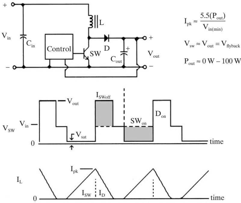
**Figure 3-10** The boost (step-up) converter.
