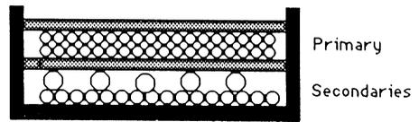
Transformer Winding Arrangement.
