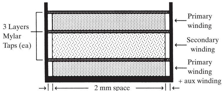
**Figure 3–68** The transformer winding technique for design example 3.15.3.
