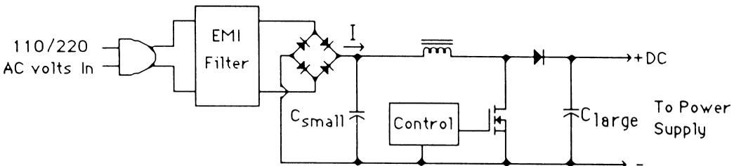
Figure C-5 A boost power factor correction circuit.
