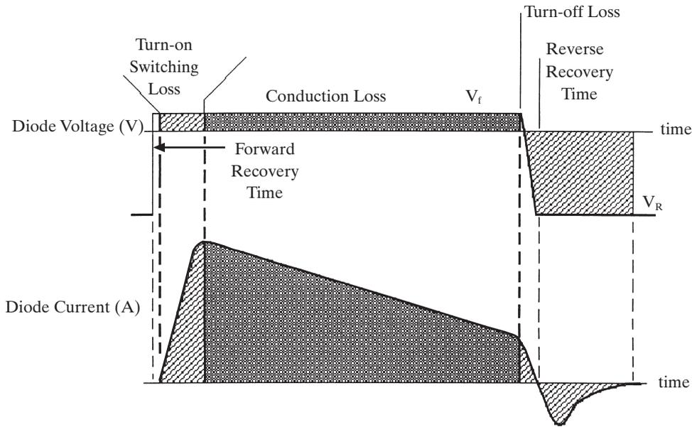
Figure 4-2 Rectifier losses.
