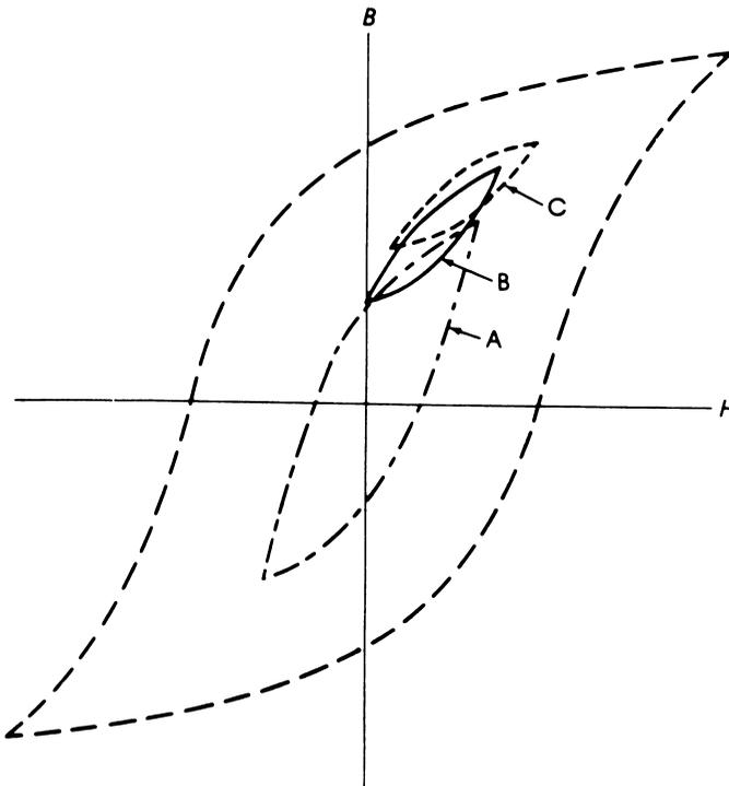
Figure D-3 Minor loop B-H curves for various magnetic components.
