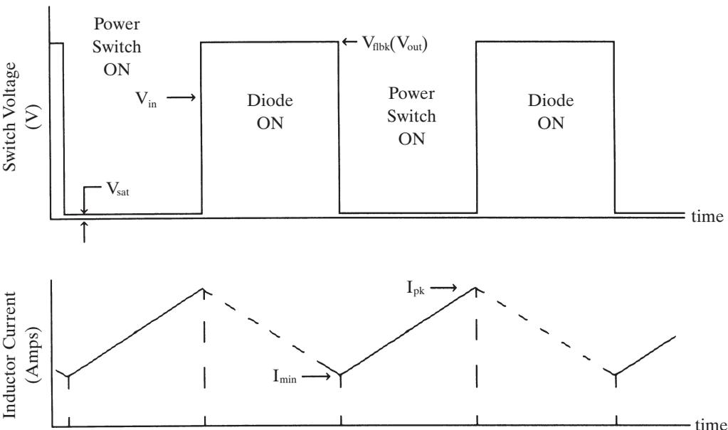
Figure 3–5 Waveforms for a continuous-mode boost converter.
