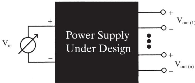
Figure 3–17 The SMPS treated like a black box.
