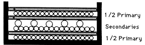
Transformer Winding Arrangement.
