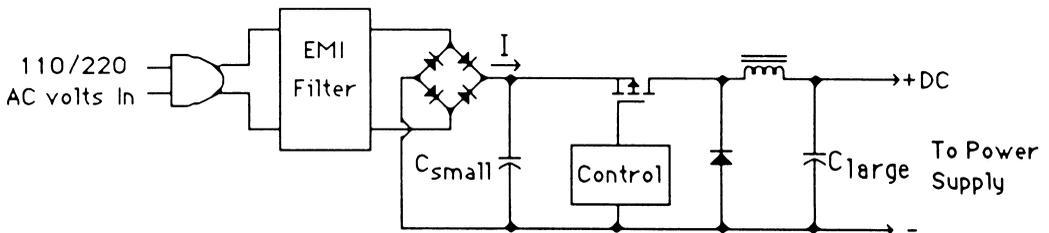
Figure C-3 A buck power factor correction circuit.
