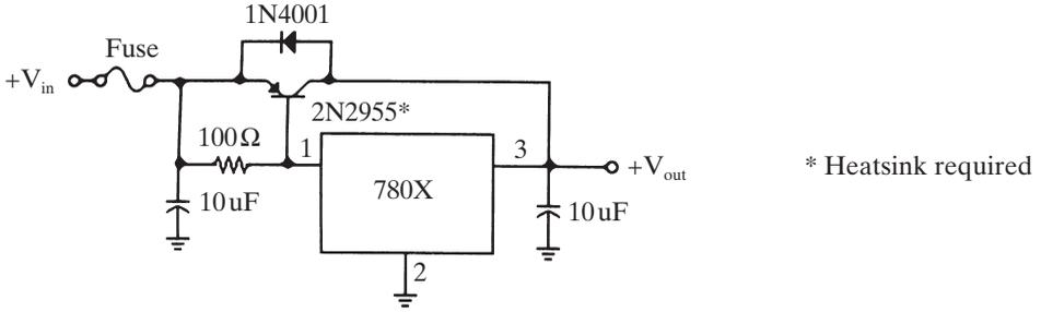
Figure 2-6 Current-boosted 3-terminal regulator without overcurrent protection.
