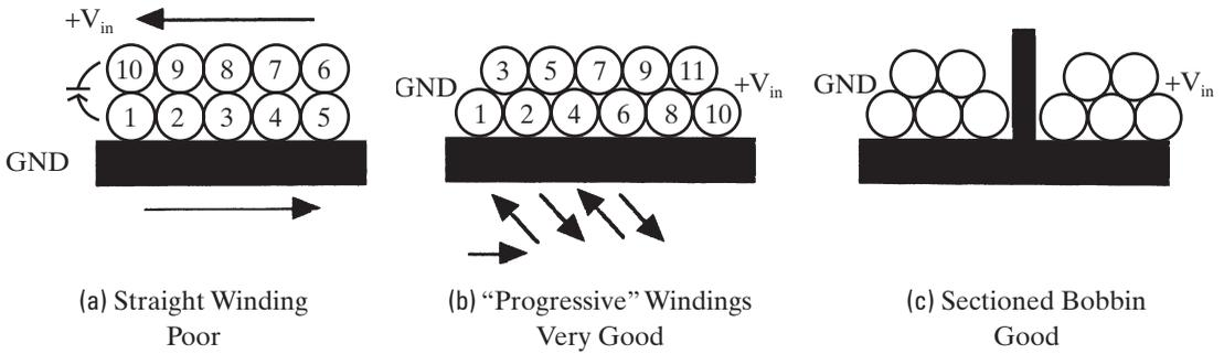
**Figure 3-26** Winding technique for minimizing inter-turn capacitance.
