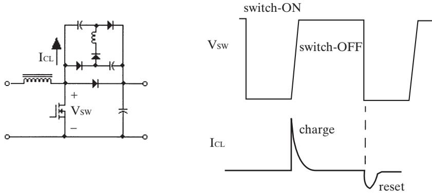
Figure 4-6 Lossless snubber for a boost converter.
