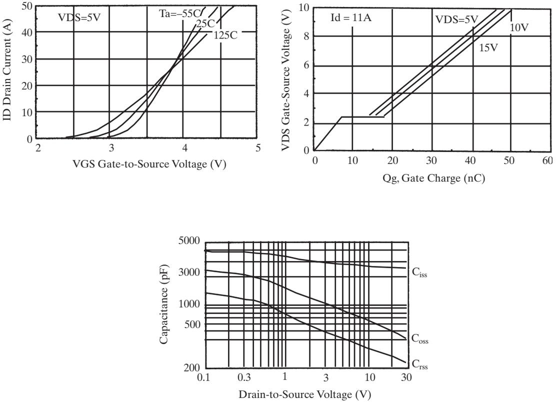
Figure 3-37 Representative datasheet curves for a MOSFET.
