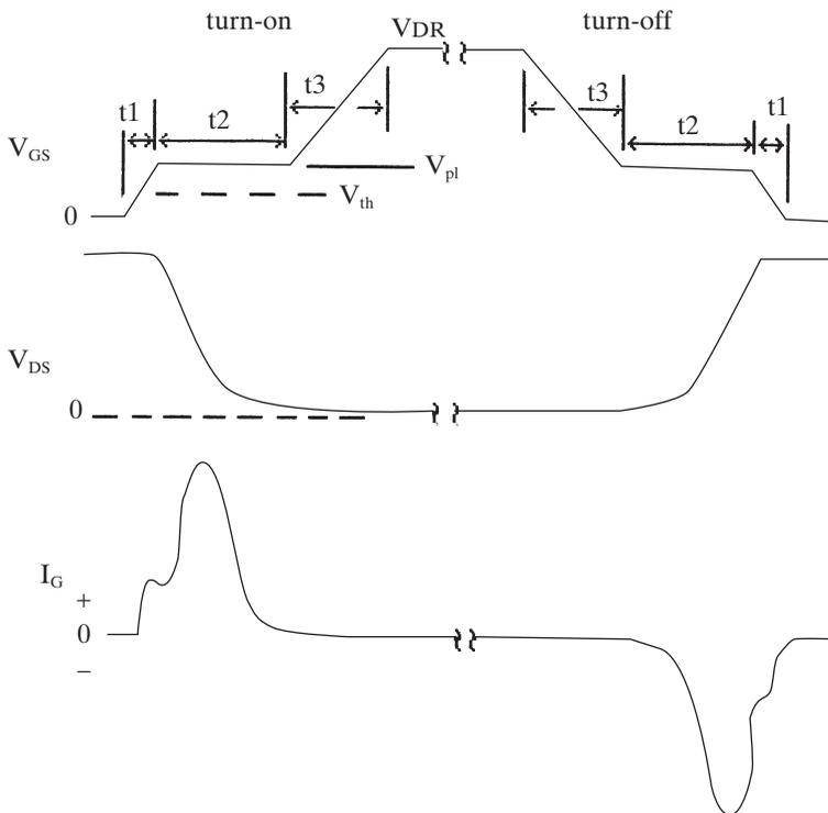
**Figure 3–36** The MOSFET waveforms.
