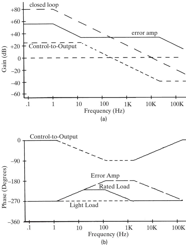
**Figure 3-71** The gain and phase plots for design example 3.15.3: (a) the gain plot for the power supply; (b) the phase plot for the power supply.
