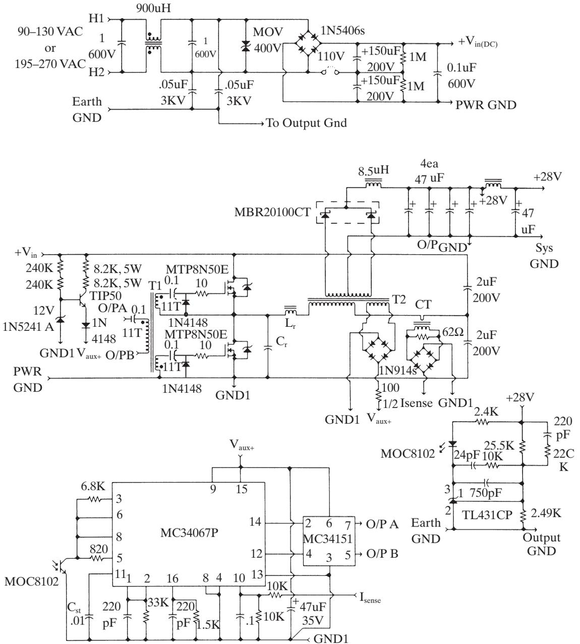
Figure 4-25 Schematic for the ZVS QR half-bridge converter.
