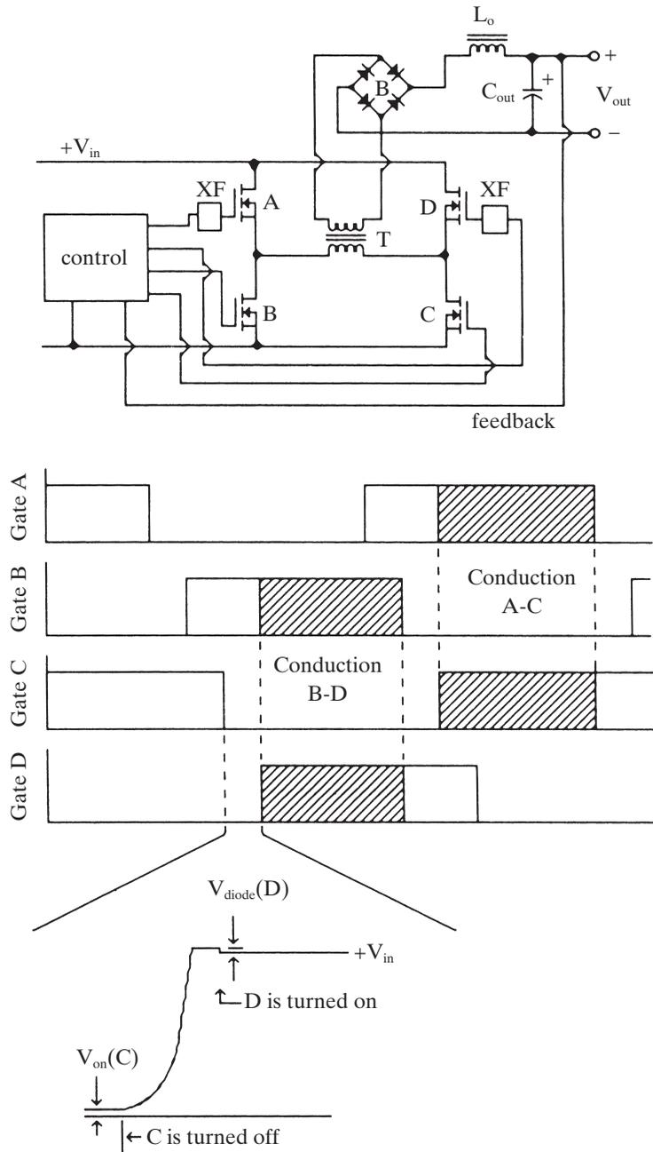
Figure 4-18 Phase modulation of a PWM full-bridge converter.
